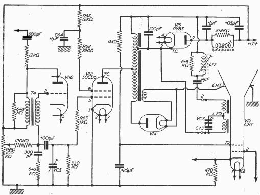
Fig. 3.—Line timebase circuit.
