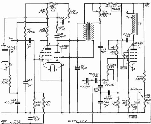
Fig. 4.--Frame timebase circuit.
