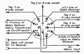
Fig. 5.—Connections to 4-pole, two-way switch.
