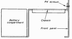
Fig. 4.—Assembly of the chassis and battery compartment.
