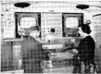
Mr. Walter Kemp, Technical Controller of TWW, loads the two-inch wide magnetic tape on to the video and audio record heads for recording in the new specially-designed mobile Ampex videotape recording unit. This unit, which has just been delivered to TWW, will be used for recording studio programmes and outdoor events in Wales and the West Country. This picture gives a close-up of the Ampex console with the record and preview picture monitors on each side of the waveform momitor.
