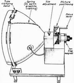
Fig. 5.—Cossor 945; chassis with cabinet removed.
