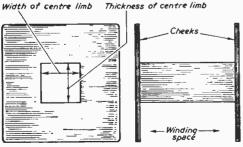
Fig. 2.—Bobbin and core size.
