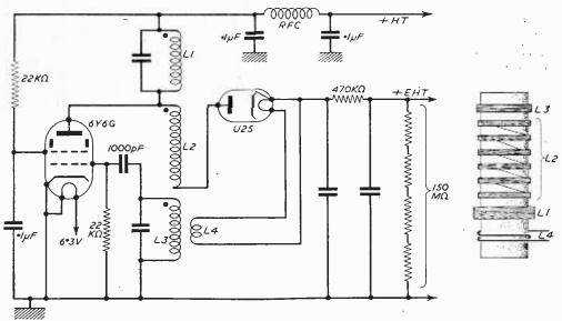
Fig. 6.—Positive R.F. EHT supply for a picture tube.
