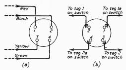
Fig. 4a (Left).—Connections to 4-pin plug (rear view).
