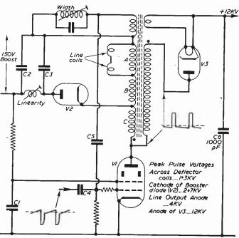
Fig. 7.—Line output stage for 17in. tube.
