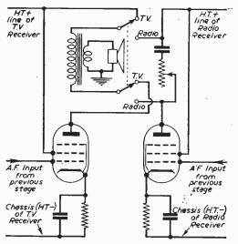
Fig. 1.—Changeover switching for feeding output transformer from TV or radio.
