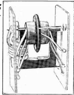
A home-constructed line-output transformer,
