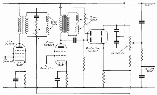
Fig. 49.—Projection tube protection circuit.
