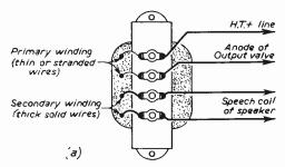
Fig. 3a.—Connections to output transformer before modification.
