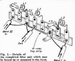
in Fig. 2. Here it will be seen that the coils are made self supporting. Tinned copper wire of 18 s.w.g. is ideal and the coils are best formed on a rod of in. diameter. Coils L1 and L2 have two turns, and coil L3 three turns; the turns should be separated approximately the diameter of the wire.
