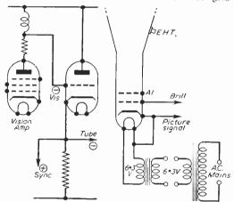
Fig. 38 (Left)—Feeding the cathode follower direct from the anode of the video amplifier. Fig. 39 (Right)—A method of using an isolating transformer in conjunction with the existing transformer.
