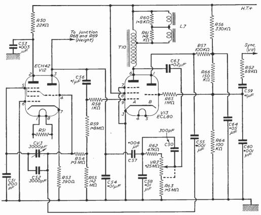
Fig. 4.--Frame oscillator and output stages.
