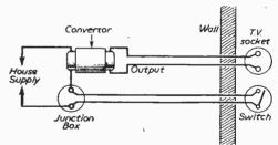
Fig. 2.—Connecting an input switch.
