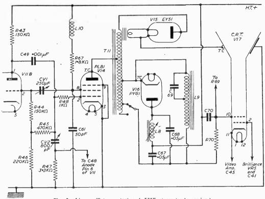
Fig. 2.-Line oscillator, output and EHT stages (early versions).
