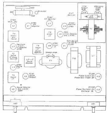
Fig. 1.-The chassis layout.
