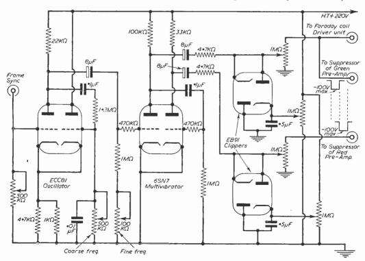
Fig. 8.—Circuit of the 25c/s double square-wave generator.
