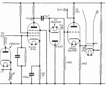
Fig. 37.—The use of two extra valves to remove the danger to the tube when grid modulation is used.
