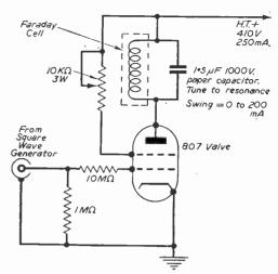
Fig. 7.—Circuit of the Faraday cell driver unit.
