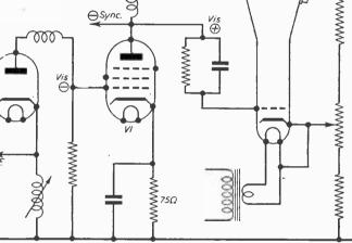
Fig. 36—Grid modulation (and the use of an isolating heater transformer).
