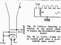
rectifier if damaged by short. In tetrode tubes a short from A1 to chassis often provokes this symptom.
