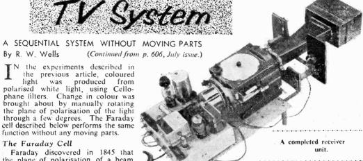
Faraday discovered in 1845 that the plane of polarisation of a beam of light was rotated on being passed through lead glass in the presence of a magnetic field. The Faraday cell consists, therefore, of an electro-magnet with
