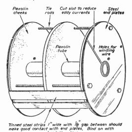
Fig. 6.—Coil former and shroud for Faraday cell. compromise between loss of light and power to be supplied to the Faraday cell.
