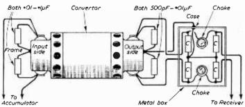
Fig. 3.—Wiring-in suppressor condensers and chokes.
