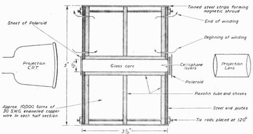
Fig. 5.—The Faraday cell as a colour switching device.
