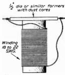
Fig. 4.—Small suppressor chokes.
