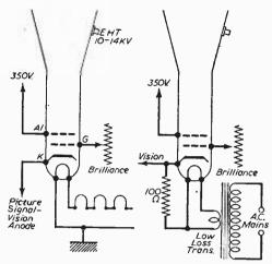
Fig. 40 (a) (Left).—Outline of circuit for a tetrode tube. Fig. 40 (b) (Right).—Using a heater isolating transformer.
