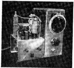
The completed generator with attached power-pack. valve pins will lie parallel to the Lecher lines—the pieces of curtain-runner—and both clips are soldered on to the same "hand" side. For soldering to the brass rail either a ½lb. soldering iron or a small blowlamp will be needed since the brass itself has a high thermal capacity
