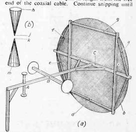
Fig. 2. — For horizontal polarisation dipole may require additional support. (a) All woodwork lin. square excepting a, b, d, e, f and g, these being lin. x \(\frac{1}{2}\)in. All joints half-lapped and screwed excepting at A and B where \(\frac{1}{2}\)in. holes are drilled and \(\frac{1}{2}\)in. dowel rod fitted. Bases of cones are plywood discs. (b) Copper strip or bonding wire around h, j, k and m to support wires. Connect coaxial cable to i and k:
