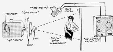
Fig. 3.—Diagram illustrating the manner in which the early television system worked.
