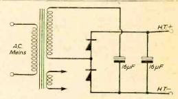
Fig. 7.—A voltage-doubler to be avoided. (50c/s ripple and poor regulation.)
