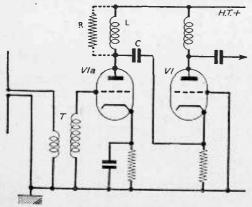
Fig. 4. — The basic cascode circuit.
