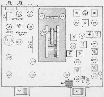
Fig. 3.—Simplified under-chassis view. Note W2 V6 bias metal rectifier, core of L32 and R82. The PL81 grid-leak is R27 2.2 MΩ. R112 may not be fitted.
