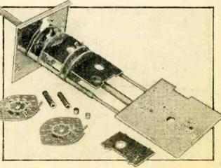
Component parts of the switch assembly
