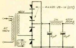
Fig. 3.—Bridge rectifier developed from the push-pull version of Fig. 2.
