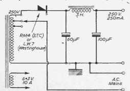
Fig. 5.—Half-wave system directly connected to mains.
