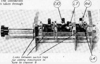
· View of the switch unit with some components identified.
