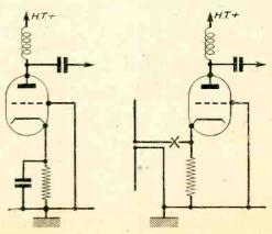
Fig. 2. - Grounding the grid.
