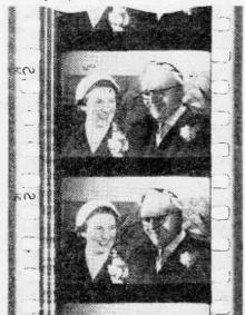
These two frames of a cinema film illustrate what is meant by persistence of vision. Although the illusion of continuous motion is provided by the film, it is really a series of stills, the film being drawn past the lens in a series of jerks.
