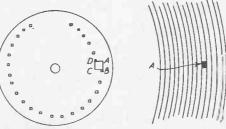
Fig. 1.—How the first type of picture was built up by a rotating scanning (perforated) wheel.
