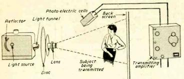
Fig. 3.—Diagram illustrating the manner in which the early television system worked.
