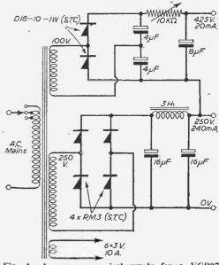
Fig. 4.—A more economical supply for a VCR97 Receiver, which can later he used for a magnetic picture tube if required.
