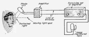
Fig. 2.—How the image was first transmitted and received.
