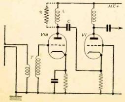
Fig. 4. - The basic cascode circuit.
