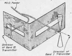
Fig. 3. — Slot length = R. Slot width =  $\frac{R}{12}$ Chicken wire extends to a distance at least  $\frac{R}{4}$  from slot. Dipoles placed  $\frac{\lambda}{4}$  from centre of slot.
