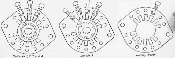
Fig. 3.—Details of the six switch wafers.
