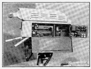
Three-tube colour camera, side view, showing one of the camera tubes in its yoke and its associated amplifiers.
