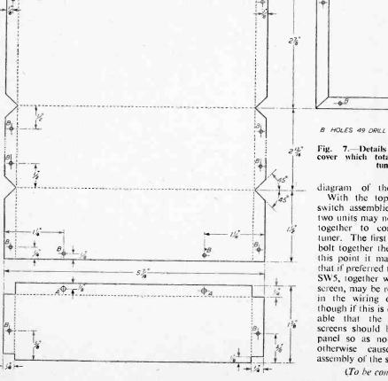
Fig. 7.—Details 'of the metal which totally encloses the tuner.
