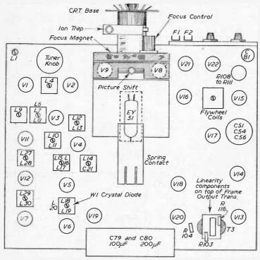
Fig. 1.—Plan view of chassis. Note position of EY51 and W1 crystal-diode
