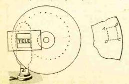
Fig. 4.—Another illustration of the method of building up an image by a mechanical disc.
