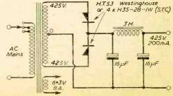
Fig. 2.—Valve replaced by a push-pull metal rectifier.
