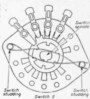
Fig. 8.—Details of the spindle earthing spring.
