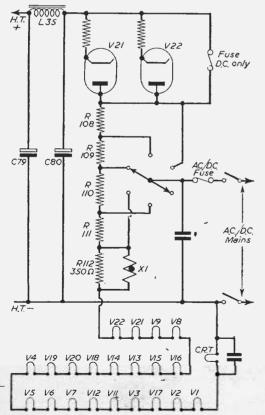
Fig. 4.—Showing power supplies and heater chain. R112 only fitted with Brimistor (X1) or Varite.
