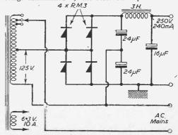
Fig. 6.—Voltage-doubler using equivalent of RM4, with more economical ripple suppression. Neither side of mains directly connected to chassis.
