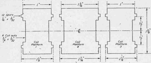
Fig. 5.—Details of the coil platforms-made from paxolin.
