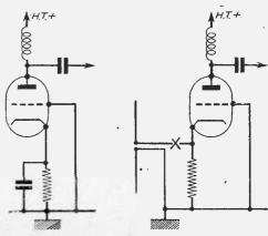
Fig. 2. - Grounding the grid.
