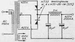
Fig. 2.-Valve replaced by a push-pull metal rectifier.
