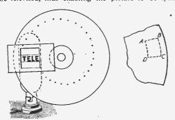
Fig. 4.—Another illustration of the method of building van an image by a mechanical disc.
