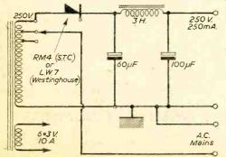
Fig. 5.—Half-wave system directly connected to mains. Boosted if below this voltage. Note the high values of the capacitors.
