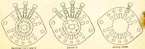
Fig. 3.-Details of the six switch wafers.
