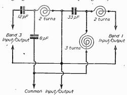
Fig. 20.—A circuit diagram of a tuned filter.
