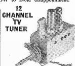
Famous make. Covers Bands I and III. Complete with valves EF80 and ECC81. Ceramic valveholders, finest quality components, precision made. Switch and fine tunion. Switch and fine tuning. I.F. output 20-25 and 40-50 Mc/s. Freq. coverage 50/87 Mc/s and 175-215 Mc/s. Supplied with full details and circuit diagram.
