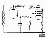
Fig. 2.—Negative grid input for grid-modulated tubes.
