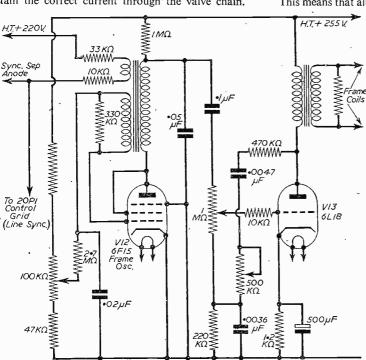
Fig. 4.—Frame Timebase and feed to sync separator,
