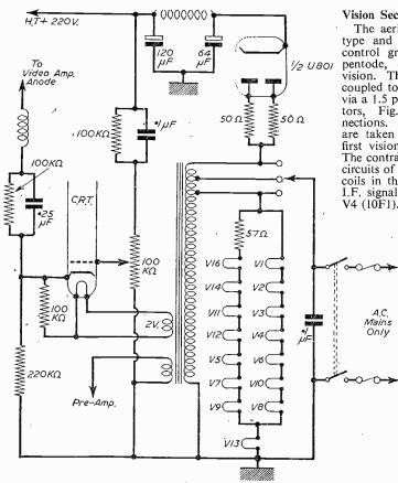
Fig. 2.—Mains circuit showing heaters and C.R.T. supply of the T161, TC162 and TC166.
