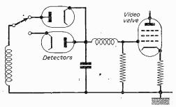
Fig. 4.—Switched grid input for positive or negative modulated carrier.
