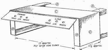
Fig. 4 (above).—Alternative arrangement for the timebase controls, which are mounted on a hinged panel at the rear.
