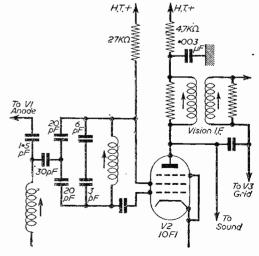
Fig. 1.—The Frequency Changer Stage.
