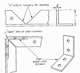
Fig. 2 (upper).—Angle aluminium used for side runners A and B. (Lower) Method of finishing off "open" ends of side runners by means of flat angle irons.
