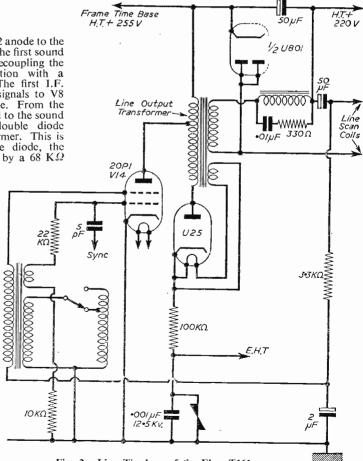
Fig. 3.-Line Timebase of the Ekco T161.
