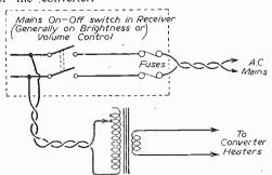
Fig. 27.-If a separate heater transformer is used the mains input should be arranged as shown here.
