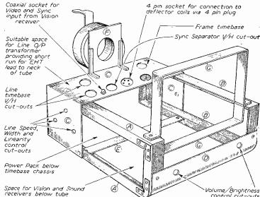
Fig. 1.—General view of the complete chassis framework.
