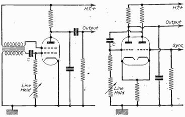
Fig. 7.—Typical blocking oscillator.
