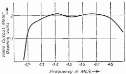
Fig. 4.—Showing how a graphic representation of an overall response curve can be obtained by plotting the generator frequency within the vision passband against the reading given on the video output indicator.
