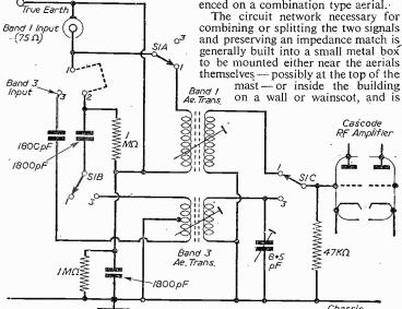
Fig. 16. - The two-band aerial input circuits used in Ferranti receivers.
