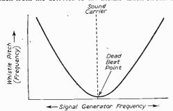
Fig. 5.—A diagrammatic illustration of the dead-beat point.
