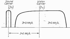
Fig. 1.—A double sideband transmission in which the sidebands extend to plus and minus 3 Mc/s about the carrier frequency (fv). Showing also the sound transmission about the sound carrier (fs).
