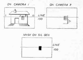
Fig. 1.—Principles of the arrangement known as 'Inlay.' The Inlay equipment described in this article is installed in several television studios and is often used for Inlay, for Wipes, and for Overlay. It is a valuable adjunct to the television service. amplified and used to operate the switch to (say) Camera 1. If the light is interrupted then the photoelectric cell current ceases and the switch changes over to Camera 2.
