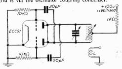
Fig. 4.—Twin triode push-pull oscillator. The coupling coil L comprises two turns wound centrally over the anode coil.
