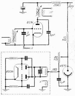
Fig. 5.—A mixer and oscillator combination with variable voltage control to oscillator (Values as Fig. 4).
