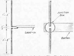
Fig. 1 (left).—Basic dipole for Band III. Fig. 2 (right).— Terminating the dipole.
