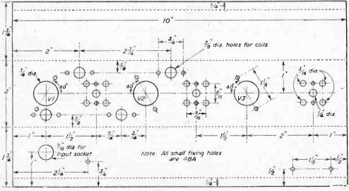
Fig. 10.-Chassis drilling data for the fringe model,
