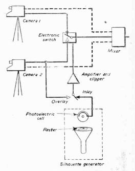
Fig. 2 .- Block diagram of the complete set-up for Inlay or Overlay.
