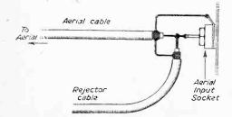
Fig. 1.-Connection of the rejector.
