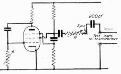
Fig. 1.-Exciting the transformer from a transitron.
