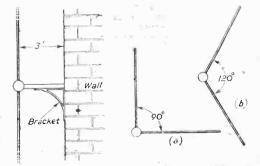
Fig. 3 (left).—Mounting the dipole. Fig. 4 (right).—" L" and " V " type dipoles.
