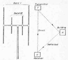
Fig. 9 (left).—A composite aerial for both Band I and Band III. Fig. 10 (right).—Reflected signals.
