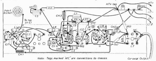
Fig. 11.—Wiring details of the fringe model.
