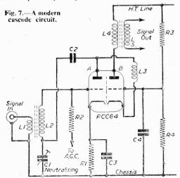
power gain in the region of four times, the "noise" produced in the following circuits and valves is negligible in comparison and can thus be ignored.
