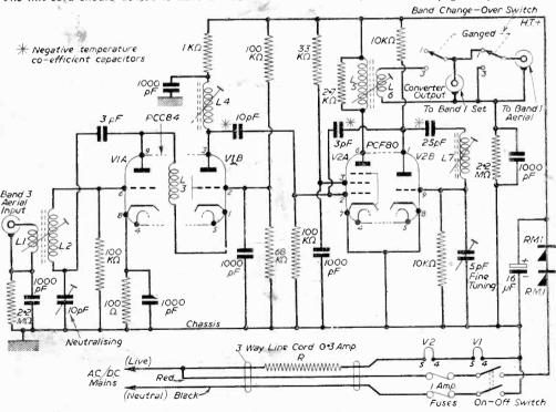
Fig. 10.-A cascode Band III converter circuit.
