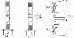
Fig. 8.—Details of the I.F. coils. (a) and (b) windings are identical.
