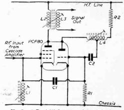
Fig. 8.-A Band III frequency changer circuit.
