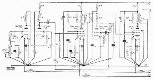
Fig. 9.-Theoretical circuit of the fringe model converter.
