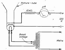
Fig. 60.—A picture-tube reactivating circuit.
