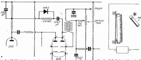
2.-Modified frame timebase with component changes. Note addition of small rectifier shunted by 2,2 M $\Omega$  resistor.
