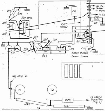
Fig. 6.—The E.H.T. and C.R.T. network.
