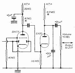
Fig. 4.—Valve-limiter circuit. The load resistor of the DH77 may be changed to 220 K $\Omega$  to minimise distortion with stressing of sibilants. Also the 4.7 M $\Omega$  resistor may be decreased to 2.2 M $\Omega$ .
