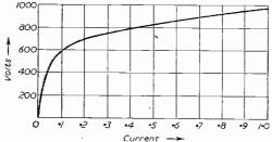
Fig. 1.—A graph showing the non-linear volt-ampere property of Metrosil.
