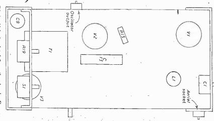
Underside and top chassis layouts for the unit. Note that C6 should be an experimental condenser and is replaced Note that C6 should be insulated from the chassis. Cx was 1 by C15.
