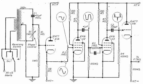
On the left is the phasing network, feeding the pulse forming circuit.
