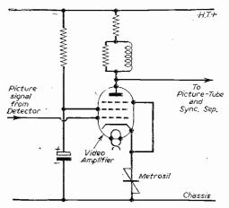
Fig. 4.—A Metrosil in the cathode circuit of a video amplifier assists in maintaining a linear response.
