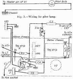
Fig. 4.—Wiring of the amplifier.
