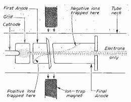
Fig. 62.—Illustrating the electron-gun assembly as used in the new Mazda tetrode tubes.
