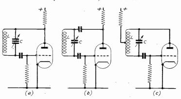
Fig. 1.—Showing (a) Colpitt's (b) Hartley, and (c) Ultraudion oscillators respectively.
