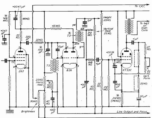
Fig. 1.—The components mentioned in the article are marked with an asterisk. Note: The component valves may be found to differ from those marked.
