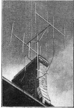
Fig. 59.—This type of double four-element aerial system is often essential for good pictures in fringe areas.
