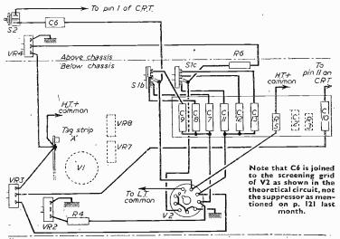
Fig. 5.-Wiring of the oscillator.
