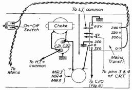
Fig. 7.—Wiring of the power supply.
