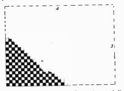
Fig. 1.—Standard raster with picture elements indicated as a check pattern.
