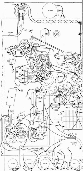
Fig. 5.-Main wiring details below chassis. §
