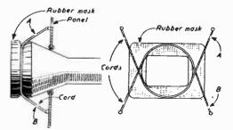
Fig. 3.-Method of mounting the mask.
