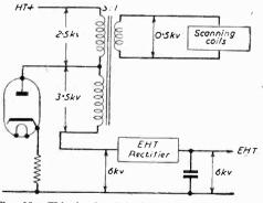
Fig. 30.-This is the flyback E.H.T. arrangement.
