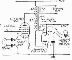
Fig. 12.-A typical line flyback E.H.T. circuit.
