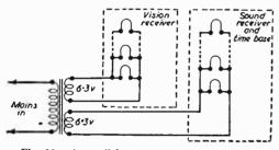
Fig. 22.-A parallel heater wiring arrangement.
