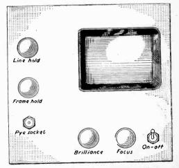
Fig. 4,-Panel layout and control positions.
