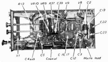
View of the completed unit. Positions of main components.
