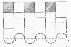
Fig. 2.—Type of wave giving the black and white pattern. One cycle is from a to b.
