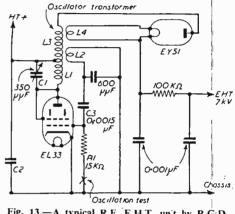
Fig. 13.—A typical R.F. E.H.T. unit by R.G.D. (Model B2 351T).
