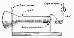
Fig. 2.—Method of mounting the tube as described last month.
