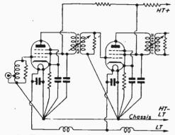
Fig. 3.—The use of double-wound coils and taking all chassis connections to one point for each stage eliminates chassis currents.
