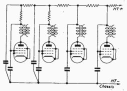
Fig. 4.—Skeleton circuit indicating the method of providing progressive H.T. decoupling.
