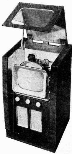
The novel cabinet, obtainable from Messrs. Tallon, which enables the tube face and protecting glass to be kept clean.
