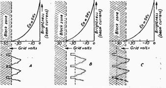
Fig. 1.—Diagrams showing the effect of picture contrast ratio for various<sup> $\omega$ </sup> brilliance settings. (a) Correct, (b) too much and (c) too little brightness.\*
