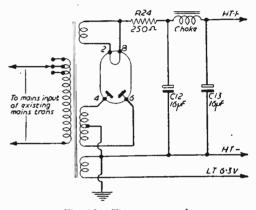
Fig. 16.—The power supply.
