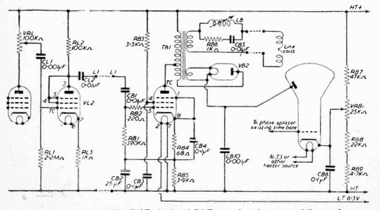
Fig. 19.-Line timebase amplifier, E.H.T. circuit and C.R.T. networks, using overwound line transformer.
