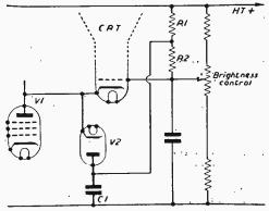
Fig. 4.—Illustrating the vision interference limiter circuit as used in certain G.E.C. receivers.
