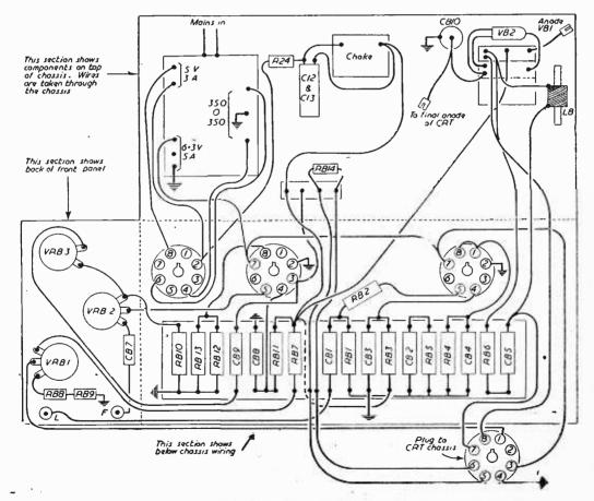
Fig. 21.-Wiring Diagram of "B" Unit.
