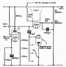
Fig. 3.—Picture-tube control circuit of the Ferguson Model 288T.
