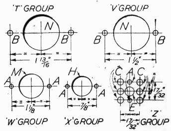
Fig. 3.-Drilling data for "Group" holes in Fig. 2 (p. 120)
