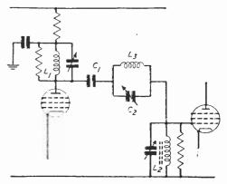
Fig. 3—Coupling using 3 coils made up as shown in Fig. 4.
