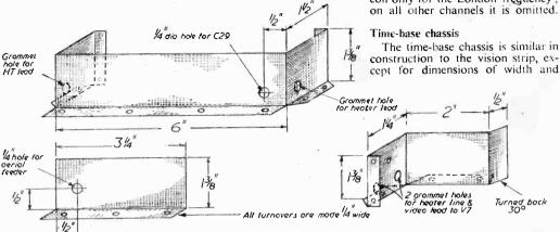
Fig. 2.—Details of the underchassis dividing screens.
