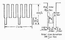
Fig. 5 (left).—One line of the suggested test pattern waveform. Fig. 6 (right).—Porch and line sync pulse details.
