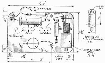
Fig. 5.—Paxolin or bakelite panel which is mounted above to carry booster and width control components.
