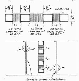
Fig. 4—Details of coil construction and mounting for the arrangement shown in Fig. 3.
