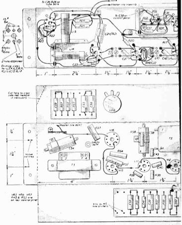
Fig. 1 (top).—Layout of the vision-sound strip, with wirings
