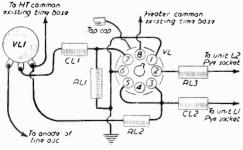
Fig. 13.—Wiring diagram of line phase-reversing circuit.
