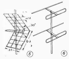
Figs. 5 and 6.—A folded dipole with 90 deg. reflector, and a stacked array of two folded dipoles with reflectors.
