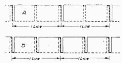
Fig. 3.—The relative timing of frame and line sync pulses.
