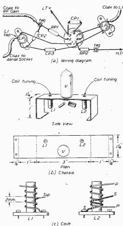
Fig. 22.—Details of the pre-amplifier and coils.
