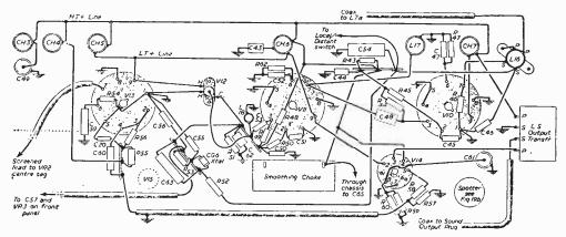
Fig. 20.-Wiring details of the sound section.
