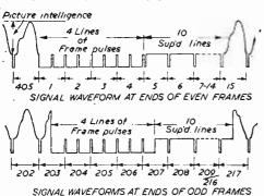
Fig. 1.—The standard BBC television waveforms.
