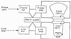
Fig. 17.—Schematic electro-magnetic deflection arrangement.
