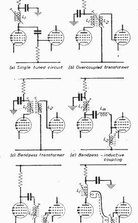
Fig. 1—The various types of interstage coupling.
