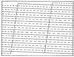
Fig. 2.—The interluced half-frames.
