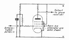
Fig. 9.—Obtaining line sync pulses,
