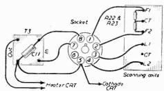
Fig. 14.—Wiring diagram of the C.R.T. chassis.
