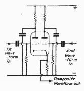
Fig. 12.—Basic waveform mixers.
