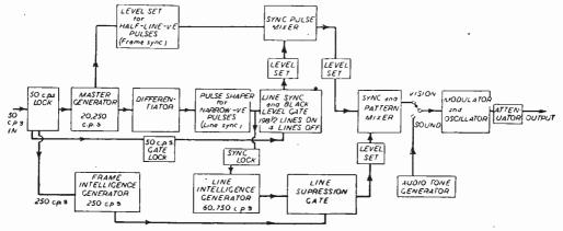
Fig. 7.—One approach to a standard test pattern generator.
