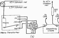
Fig. 21.—Wiring details of the power pack (a) is for a VU39A and (b) for a 5U4G.
