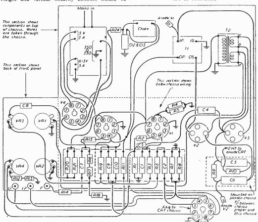
Fig. 15.-Wiring diagram of the unit.
