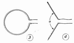
Figs. 3 and 4.—A circular and a "V" aeriat. The angle  $\theta$  may be varied to find the most suitable one for the receiver and locality.
