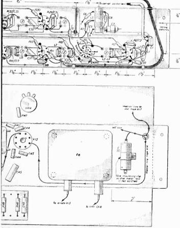
and Fig. 4 (below). - Main details of the time-base chassis.
