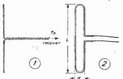
Figs. 1 and 2.—A dipole made from ordinary lighting flex and a folded dipole. L and W may be varied to find the best combination.
