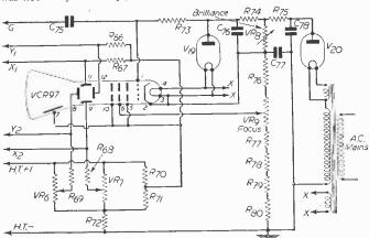
Fig. 6.-Circuit of the CRT network.
