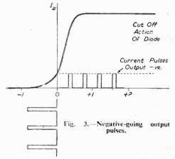
modify the circuit so as to work the amplifier on the upper bend of its curve instead of the lower bend, thus producing negative pulses at the anode of the amplifier.
