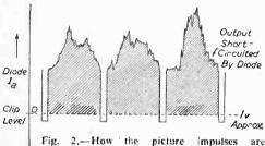
2,-How the picture impulses shorted and the negative pulses obtained,
