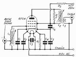
Fig. 1.—Circuit of the pre-amplifier.
