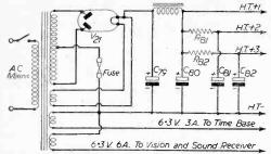
Fig. 7.—Circuit of the power pack.
