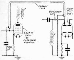
Fig. 3.—How to suple the I.F. stages of a video receive to a radio set.
