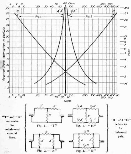
Figs. 1 & 2.—Nomograph for the design of "T," " $\pi$ ," "H" and "O" attenuators with input and output impedance of 80 $\Omega$  for use with television aerials.
