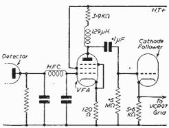
Fig. 22.-A complete video output stage.
