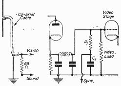
Fig. 1.—Coupling sound and vision receivers.
