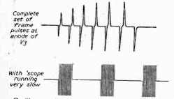
Oscillograms in connection with Interlace Filter.
