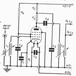
Fig. 2.—Circuit of the first R.F. stage.
