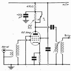
Fig. 2.—Sensitivity switch connections for parallel circuit (tuned grid).
