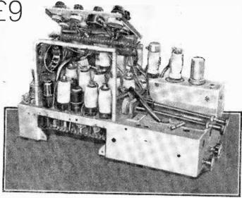
The receiver with tube removed.
