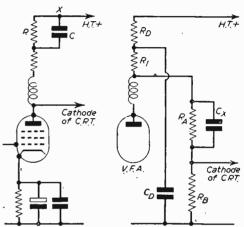
Fig. 20 (left).—L.V.F. Compensation for cathode bias circuit. Fig. 21 (right).—L.V.F. Compensation for decoupling, etc.
