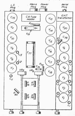
Fig. 1.-Layout of chassis top.
