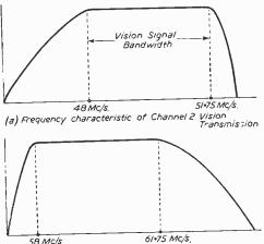
(b) Frequency characteristic of the converted Channel 2 Transmission as applied to a Channel 4 Receiver
