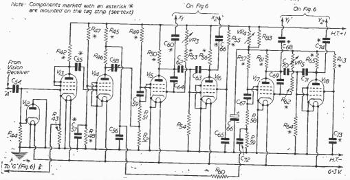
Fig. 4.—Circuit of the time-base section.
