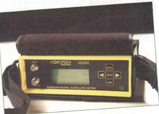
The Horizon HDSM digital satellite meter
