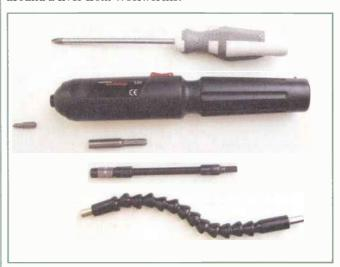
Below the power driver are some useful extensions for getting the driver bit into tricky and otherwise inaccessible spaces, partcularly when using a mini tower case as we will be doing here.
