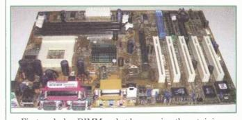
First, unlock a DIMM socket by pressing the retaining clips outwards. The align a DIMM on the socket such that
