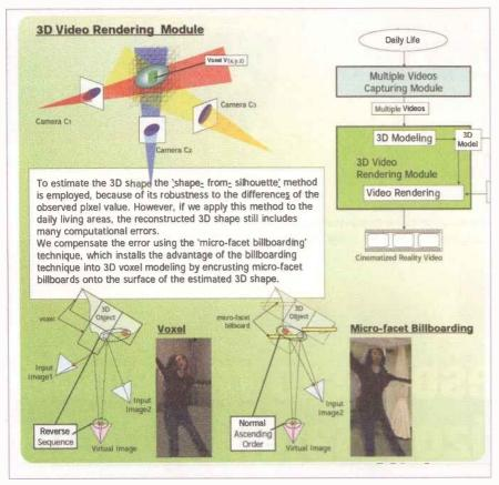
Eight portable Pentium-M 1.4-GHz PCs are used to capture a video stream from each camera and segment objects at 20 frames per second (fps). A colour-based background subtraction method is used to segment the foreground and background regions in the input multiple images.
