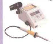
Adjustable by a potentiometer with Digital read out
