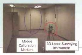
We set up multiple environmental cameras on the wall and the ceiling to surround the target object capturing almost the same area. All cameras are calibrated by combining mobile calibration markers and a 3D laser-surveying instrument.
