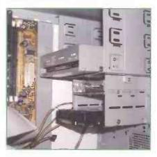
Note the position of the sockets on the various drives. The IDE drives (hard disk and CD) have sockets for power supply cables to their right as shown above, and for the IDE ribbon cables to their left.
