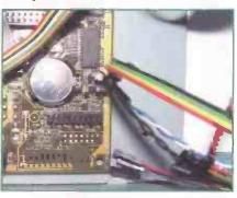
The most important convention to observe on most connections is that of the black or white cables going into the earth or ground or negative (-) pins, while just about any other colour will signify a power, signal or positive (+) pins.
