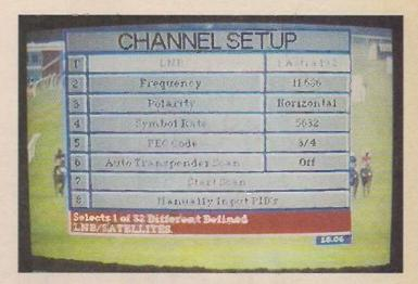
Channel set-up information from the RSD ODM-300 digital receiver, with horse racing via Eutelsat II F3 in the background.
