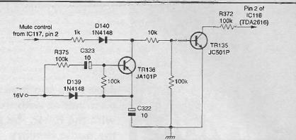
Fig. 4: Muting and anti-plop circuits used with the TDA2616 audio output chip. TR135 is switched on by the microcontroller chip IC117 to provide muting. TR136 is normally off, with 16V at its base and emitter. At switch off D139 is reverse biased and TR136's base is driven negatively. It switches on, applying the charge held by C322 to the base of TR135 which switches on to mute the audio chip.
