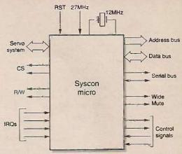
Fig. 17: Connections to a chip that combines the syscon microprocessor and gate-array functions.
