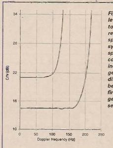
Fig. 2. Extreme levels of carrier-to-noise response for specific receiver systems at specific signal configuration indicating in general the differences between the first and second generation chip sets.
