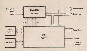
Fig. 16: Block diagram of the syscon section of a DVD player.
