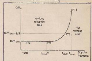
Fig. 1. Key response of carrier versus noise with doppler frequency, which can be used to define the limits of mobile reception.
