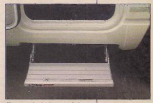
The motorised step extended while the motor home is stationary.
