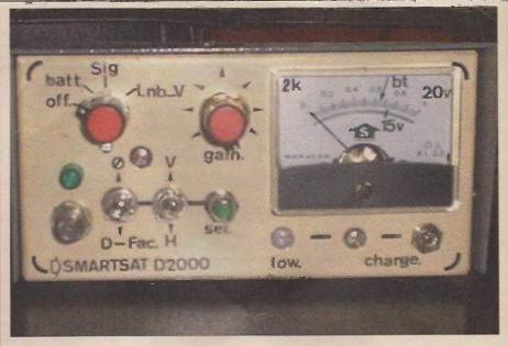
ing (or bandswitching where required). If a short is detected across the output, the meter shuts down. There's a low-battery warning LED, and the meter can be switched to check on battery condition.
