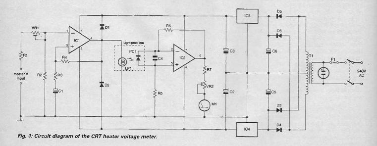
at the input. It's configured as a full-wave rectifier and is a high-power type to drive a lamp, LP1.
