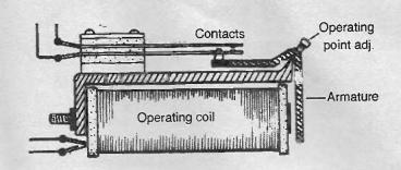
Fig. 1. PO3000 – the most common relay, as used in telephone exchanges across the world.
