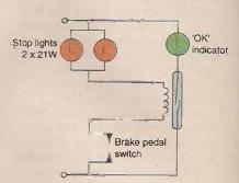
Fig. 8. This simple application of a reed switch gives the driver of a car an indication of whether or not his or her brake lights are working.
