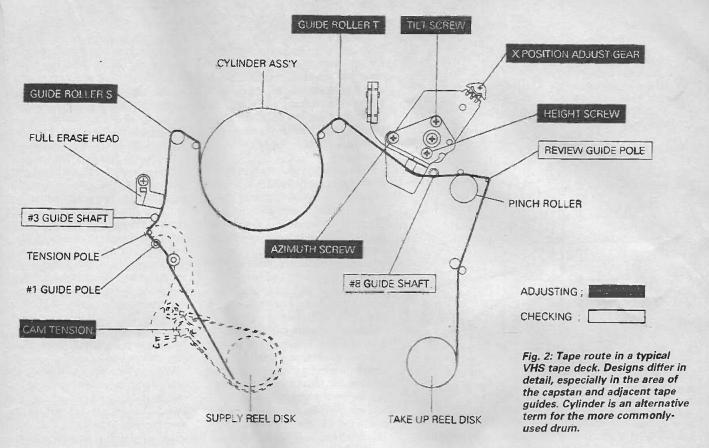
If the back-tension pole is not perfectly vertical the tape will ride up or down it. The result is tape crinkling or an incorrect tape path across the full-erase head to the drum-entry guide. The only effective way of dealing with this is to fit a new lever assembly.
