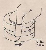
Fig. 9: Video head cleaning by hand. Keep the forefinger, wrapped in fine chamois leather, still while using the other hand to rotate the drum anticlockwise.
