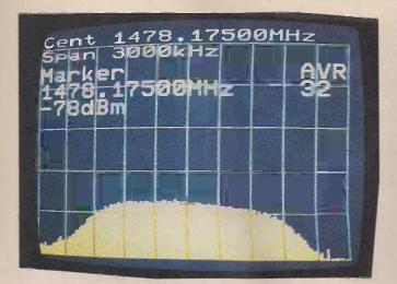
Photo 1: Afristar beam 1 spectrum for right-hand polarised signals. To take this photograph the signals from the aerial were split between the receiver and a signal analyser. Photo taken in Portugal.
