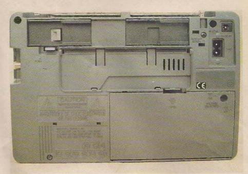
Photo 6: Rear view of the Hitachi Model KH-WS1. The mains and 6V DC input sockets are at the top right. The mains voltage adjustment is in the hole at the top, right-hand side of the battery compartment cover. The frame aerial slide/clip-in fixing lies horizontally along the top of the receiver, just below the telescopic aerial. The F input socket can be seen at the left-hand side.
