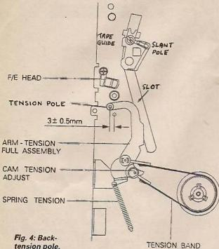
rig. 4: Backtension pole, band and setting arrangement (cam tension adjust). Note the setting indication by the pole.
