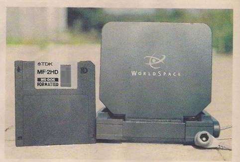
Photo 5: Close-up view of the WorldSpace aerial, alongside a standard floppy disc to give an indication of size. The flying lead from the aerial is connected either directly to the receiver's F socket or indirectly via an extension coaxial cable.
