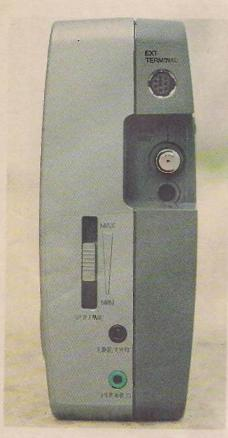
Photo 4: Side view of the Hitachi Model KH-WS1, showing the slider volume control, the line and headphone output jack sockets (bottom), the F input socket for the L-band aerial and the data socket (top).
