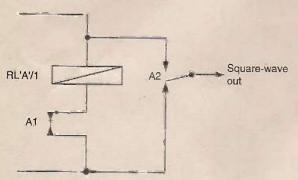
Fig. 5. Not far removed from the simple buzzer circuit, this one produces a square wave whose amplitude is equal to the supply voltage.
