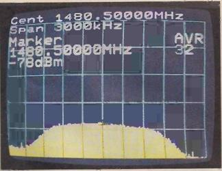
Photo 2: Afristar beam 1 spectrum for left-hand polarised signals. Conditions as for Photo 1. In the UK the left-hand polarised signals are slightly weaker than the right-hand polarised ones.
