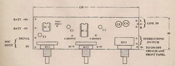
Fig. 4: Positions of the main components and connections on the stripboard. This is a suggested guide for the upper (component) side. Use the front panel as a template to position the potentiometers. Cut the potentiometer shafts to 9mm and enlarge the holes for the potentiometer legs to 1mm.
