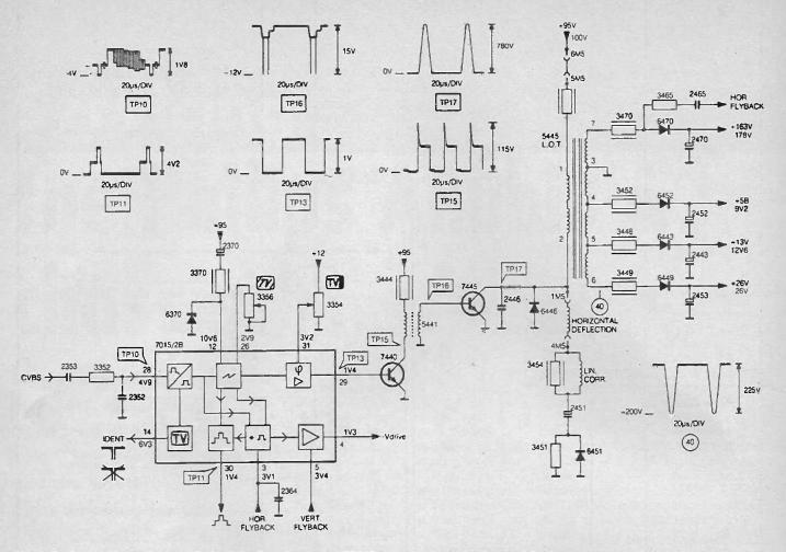
Fig. 2: Basic circuit, much simplified, of the line timebase. IC7015 contains both the line and field generators, with line drive output at pin 29 and field drive output at pin 4. It also contains the IF strip. Illustration courtesy of Philips Service.
