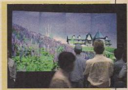
This slimline video wall system has been added to Mitsubishi's range of video appliances. The display is based on Texas Instruments' digital light-processor chip, which provides XGA quality. Control is from a PC via an RS232C port. The light-source lamp has a life of 8,000 hours and provides a high-brightness display at 500cd/m².
