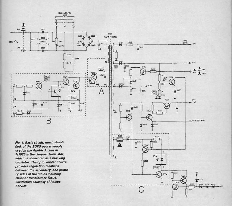
microcontroller chip IC7600. When the set is switched on, IC7600's reset pin 33 has to be kept low for at least 1msec. Zener diodes D6562/65 and transistor Tr7563 provide the reset action.
