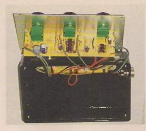
Internal view of the preamplifier/mixer unit.
