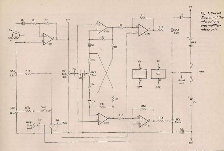
To do this correctly, the gain in one direction has to be increased by the same amount as the gain in the other direction is reduced.
