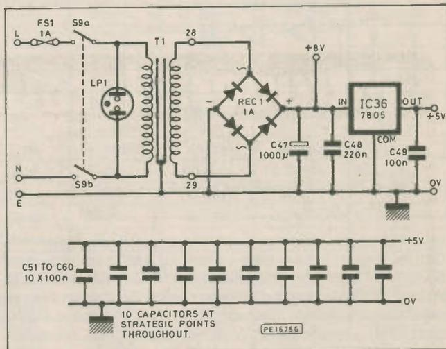
Fig. 8. Circuit diagram of the p.s.u.
