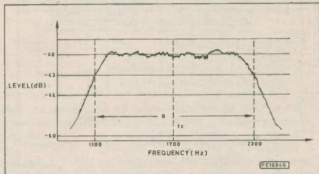
Fig. 12. V.23 spectrum at 1200 Baud
