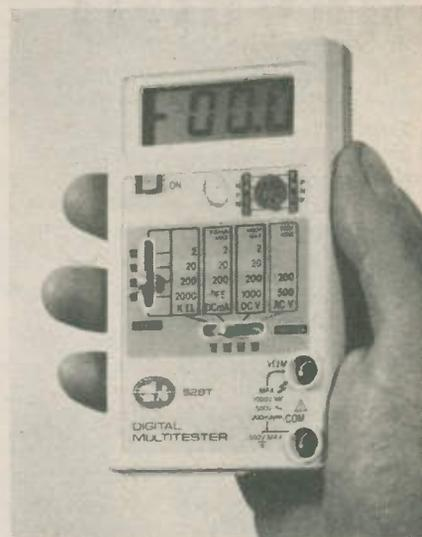
The availability of a very handy, 3½ digit multimeter has been announced by SSI Ltd. The 528T has a built-in transistor tester and measures just 115 × 65 × 24mm. Automatic zero and polarity adjustment are featured along with overload circuit protection.
