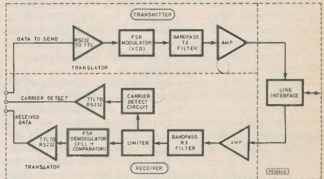
Fig. 2. Basic modem elements
