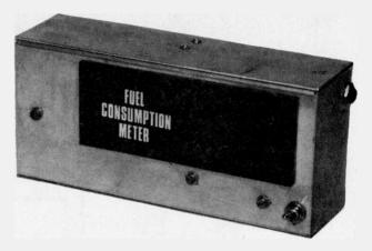
The use of a metal case is advisable for effective screening; the 5V regulator can then be mounted on the rear of the unit for excellent cooling. The driver will probably be most curious about the fuel consumption reading when accelerating hard; a time when increased concentration on the road is required, and so care should be taken in the use on this instrument.
