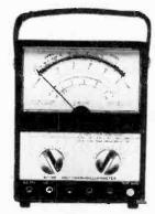
K1400 Multimeter 20,000 OPV. DC and Ar? volts up to 5000. DC and AC amps up to 10. Resistance up to 20 megohms. "Off" damping. Overload protection. R.R.P. £68.00 ex. VAT.
