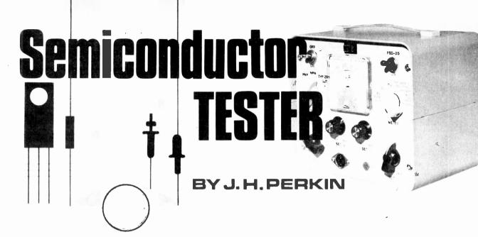
The semiconductor tester is an invaluable aid to the experimenter since it allows him to not only detect faulty components in both building and servicing but to select or match components for specific circuit requirements and, bearing in mind the availability of untested components, purchase and sort such devices.
