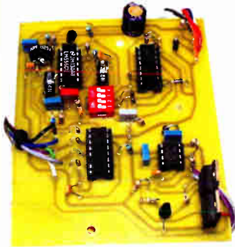
Fig.4. PCB component layout and interwiring to off-board components. Note the neon tube LP1 is glued inside the body of an old LED indicator. The annotations on the mains transformer are for the conventional primary and secondary windings.
