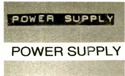
Fig.2. The label from the Dymo Mini (top) is not as good as one from an electronic labelling machine (bottom). Results are adequate though, and can be improved if due care is taken when stamping the letters and handling the tapes
