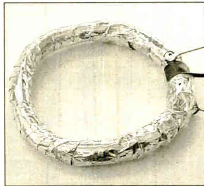
Tin-foil Faraday shield, awaiting final covering of insulating tape
