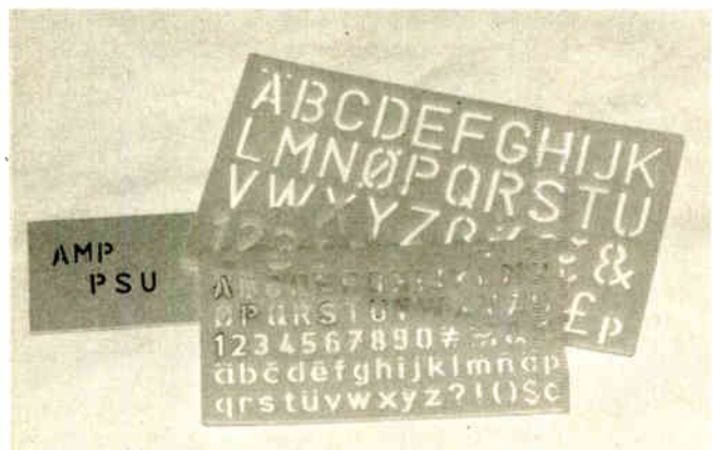
Fig.3. Using stencils it is possible to add lettering direct to a panel. Small lettering is not a practical proposition though
