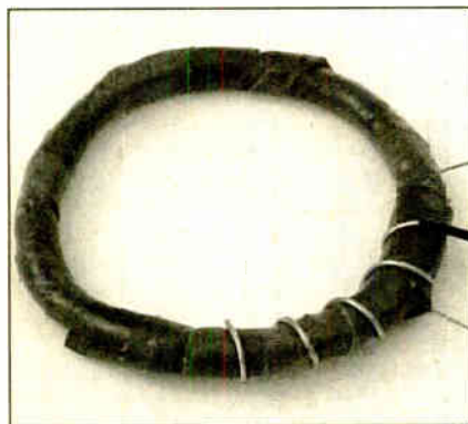
Taped-up coil and the Faraday shield awaiting final connecting wire
