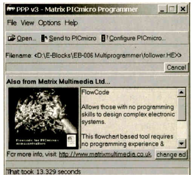
Fig.4. Running the PPP program produces this small window. Operating the Open button enables a program file to be loaded
