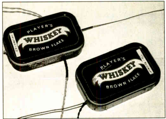
The receiver and transmitter p.c.b.s housed in ancient tobacco tins. The tins should be lined with insulation tape to avoid any "short circuits" across the copper tracks.
