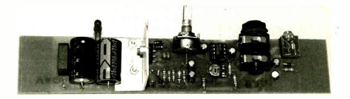
This is arranged so that inserting the headphone jack plug automatically disconnects the speaker. It also switches in a resistor, R11, in series with the headphones to prevent overloading, see Fig.1 and Fig.3.
