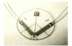
Example of a dual strain gauge module.
