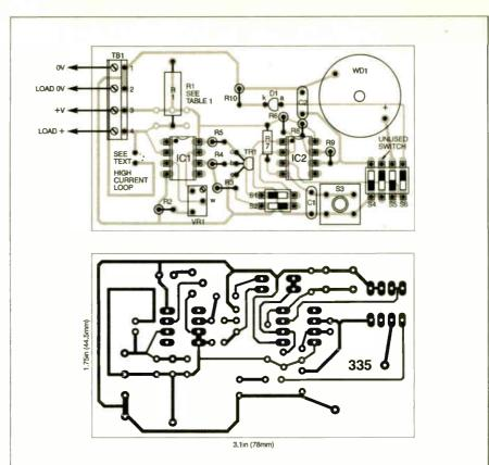
Fig.2 (above). Printed circuit board component layout and full-size copper foil master. The completed board is shown in the photograph. Allow the external circuit (load) to operate normally. The buzzer and l.e.d. may be operating already. Adjust preset VR1 until the critical point is reached. If the switching point is not sharp (the buzzer "chirps" at the threshold value), it may be necessary to improve the degree of smoothing of the supply. In most cases, however, it will not matter.
