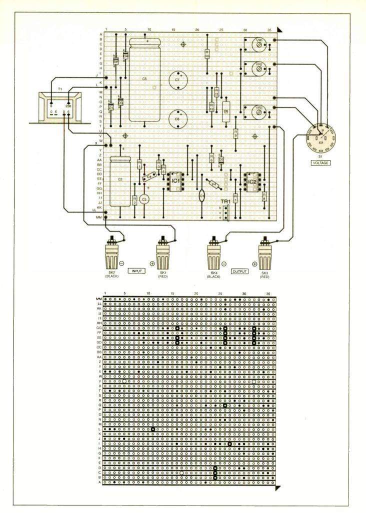
Fig.4. Stripboard topside component layout, interwiring and details of underside copper track breaks.
