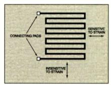
Fig.4.14. Layout of a typical strain gauge
