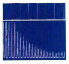
Fig.4. Amplified display of square wave harmonics.
