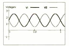
Fig.4.8. 2V peak-to-peak differential signal with 1.5V common mode voltage.
