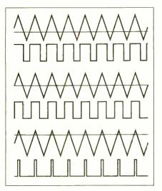
Fig.2. Example pulse width modulation (p.w.m.) waveforms.
