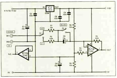
Fig.5. Circuit diagram for analogue signal pre-conditioning "front-end".
