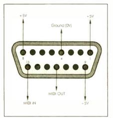
Fig.1. The pin functions of the game port when it is used as a MIDI interface.
