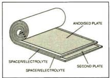
Fig.2. Construction of a traditional aluminium electrolytic capacitor.
