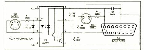
Fig.3. Circuit diagram for the MIDI Input and Thru interfaces. IC1 is a sensitive, high speed split-Darlington opto-isolator.
