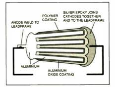
Fig.3. Construction of the new electrolytic capacitors.
