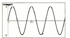
Fig.4.1. A signal varying around 0V. The peak value is 2V and the peak-topeak value is 4V. The frequency is 2.5kHz. There is no noise or error present, although the digitised sampling steps are apparent.
