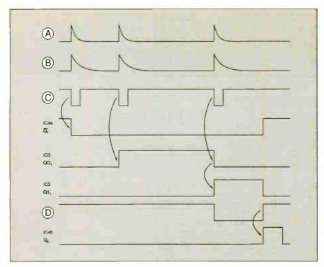
Fig.4.19. Timing waveforms for the circuit in Fig.4.18.
