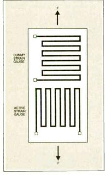
Fig.4.15. Using a dummy strain gauge for temperature compensation.
