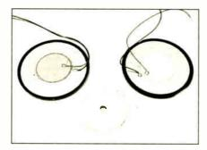
Examples of piezo sounder elements. The outer two need an external oscillating signal. The centre one is selfcontained with its own oscillator circuit.
