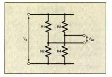
Fig.4.9. Basic Bridge Circuit
