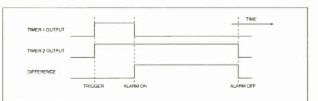
Fig.2. Circuit timing diagram.
