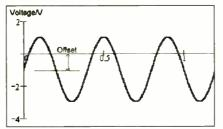
Fig.4.2. The signal from Fig.4.1 with a –1V offset. If you consider the signal rather than the offset the true peak value is still 2V, even though the signal "peaks" at +1V and –3V.
