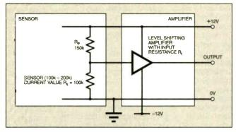
Fig.4.11. Sensor and amplifier.
