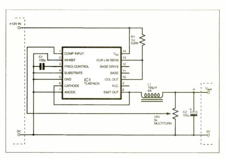
Fig.4. Circuit diagram for an In-Car Power Supply for a "Walkman" type cassette player.
