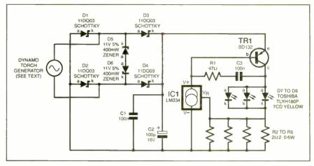
Fig.3. Circuit diagram for a L.E.D. Dynamo Torch.
