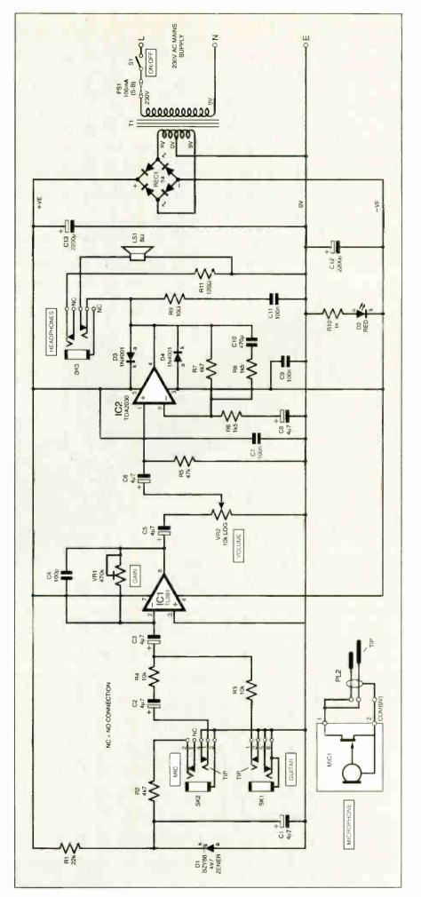
Fig.1. Complete circuit diagram for the Guitar Practice Amp.
