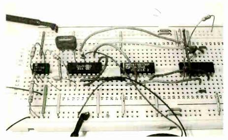
Above: Breadboard layout for the circuit in Fig.4.18. Below: Sensors connected to the above layout.
