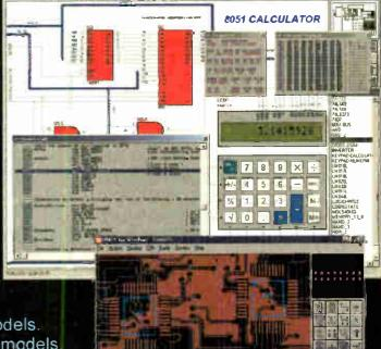
\*E.g. PROTEUS VSM can simulate an 8051 clocked at 12MHz on a 300MHz Pentium II
