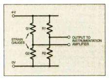
Fig.4.16. Strain gauge circuit.
