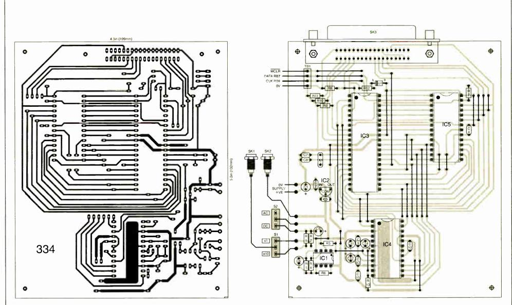
Fig.7. Component layout and full-size underside copper foil master track pattern for the PIC Spectrum Analyser.
