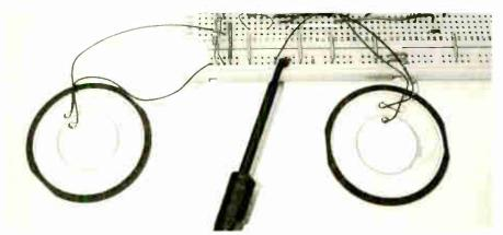
It is relatively straightforward to build this circuit on a long solderless breadboard, provided you work methodically through the circuit. Use fine long-nose pliers as necessary to help insert wires.
