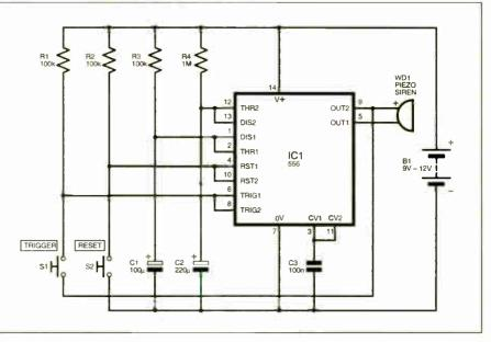
Fig.1. Circuit diagram for the Smart Alarm Timer.
