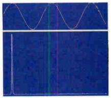
Fig.2. Analysis display for a pure sinewave.
