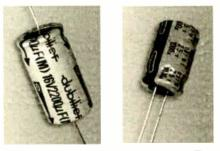
Two examples of electrolytics. The axial type (left) has "arrows" pointing to its negative (-) end. The radial type (right) has a band or arrows on one side to indicate its negative (-) lead. Some electrolytics indicate their positive connection with a plus (+) symbol.
