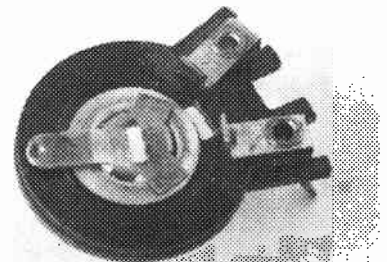
Fig.4. "Open-track" preset potentiometer.
