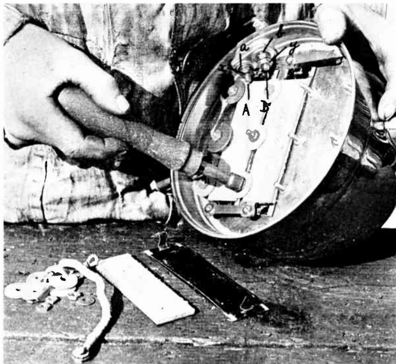
Fig. 2.—REPLACING A HEATING ELEMENT IN AN ELECTRIC KETTLE. (Sunray Tricity.)
