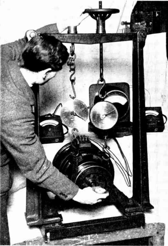
Fig. 4.—BAND BRAKE AND TESTING STAND FOR SMALL MOTOR.
