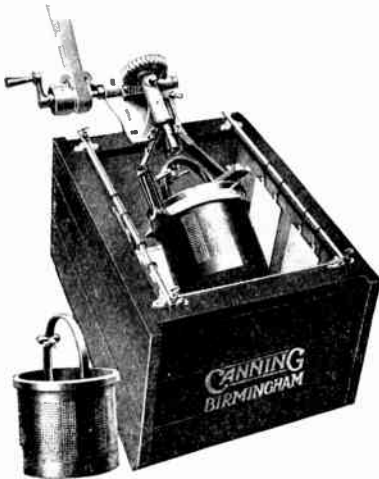
Fig. 7.—"MIDGET" PLATING APPARATUS. Suitable for mixed loads of work.
