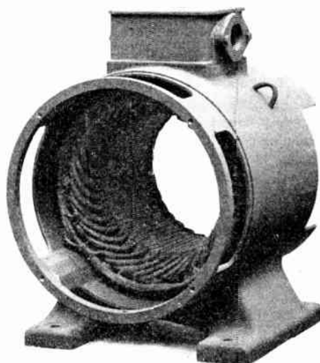
Fig. 3A.—COMPLETE STATOR OF COMPENSATED INDUCTION MOTOR. (English Electric Co.)
