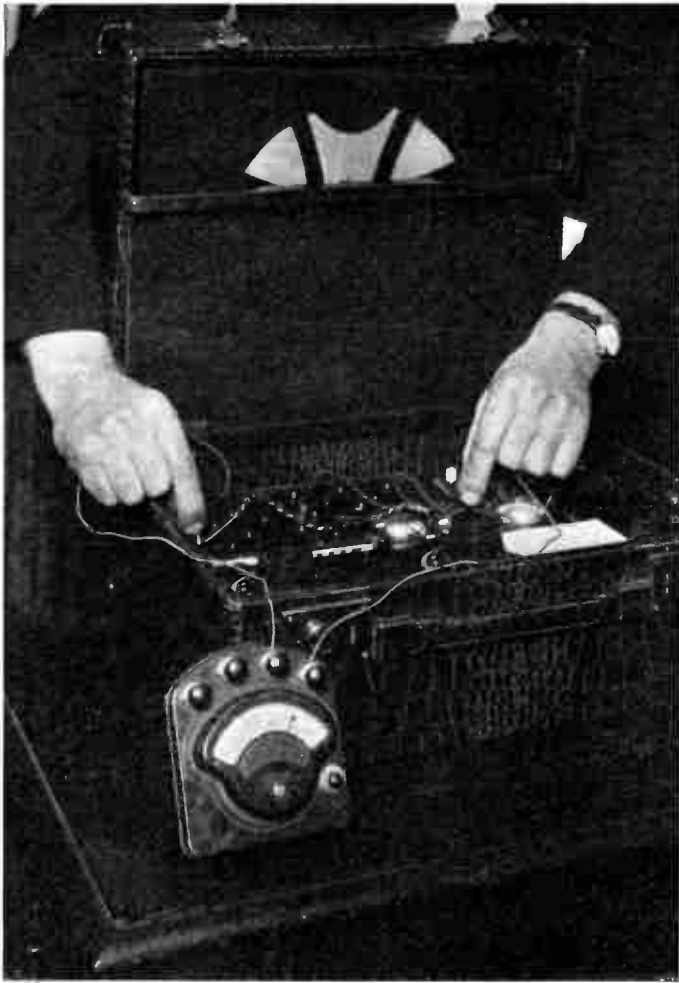
Fig. 8.—TESTING THE HIGH-TENSION BATTERY WHILE THE SET IS IN OPERATION.
