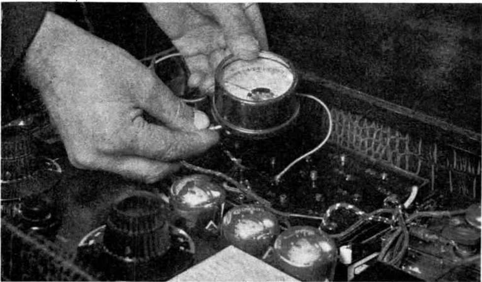
Fig. 5. —TESTING THE CONDITION OF A VALVE WITH A MILLIAMPERE METER IN THE ANODE CIRCUIT.
