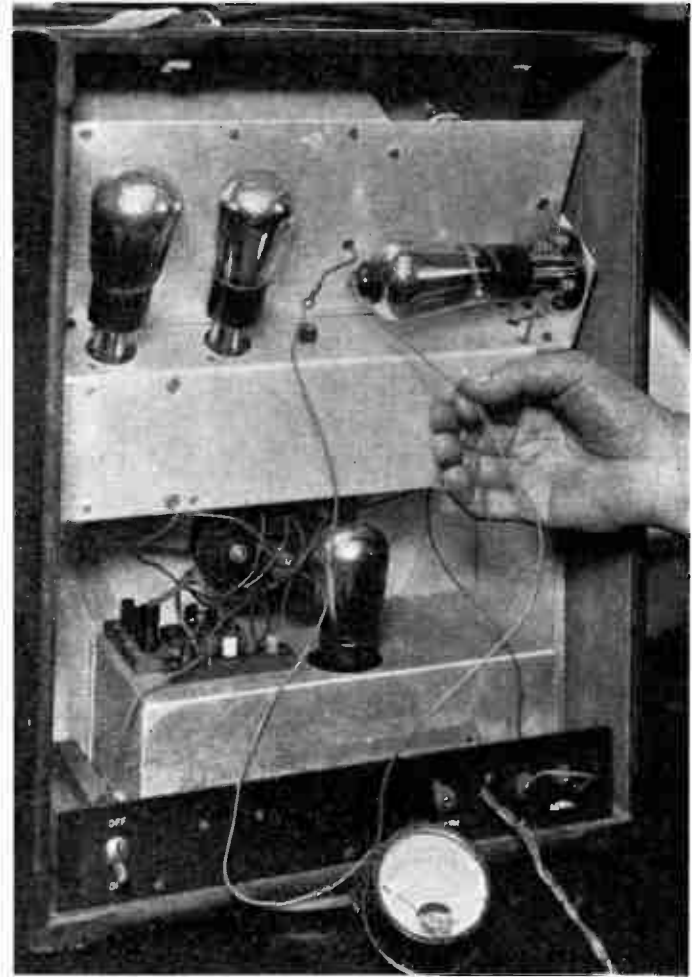
Fig. 9.—HOW TO TEST THE ANODE CURRENT OF A SCREEN-GRID VALVE.
