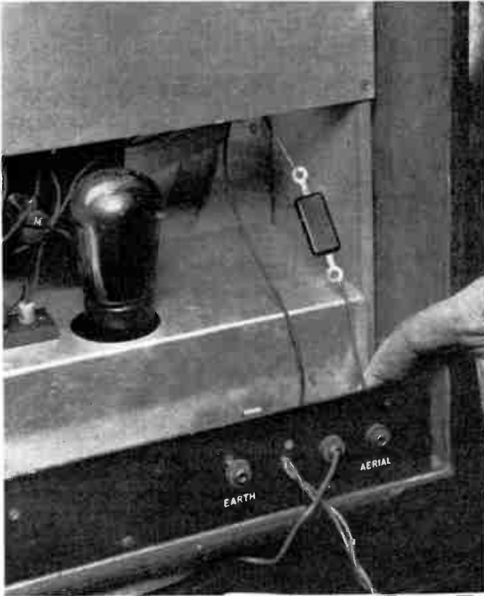
Fig. 6 (left).— PLACING A FIXED CONDENSER INSIDE THE SET FROM THE AERIAL TERMINAL.
