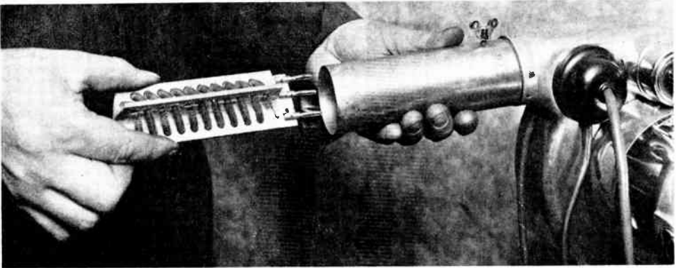
Fig. 8. —HOW TO REMOVE THE HEATING ELEMENT. All that is necessary is to give it a pull and it will come off the nozzle.
