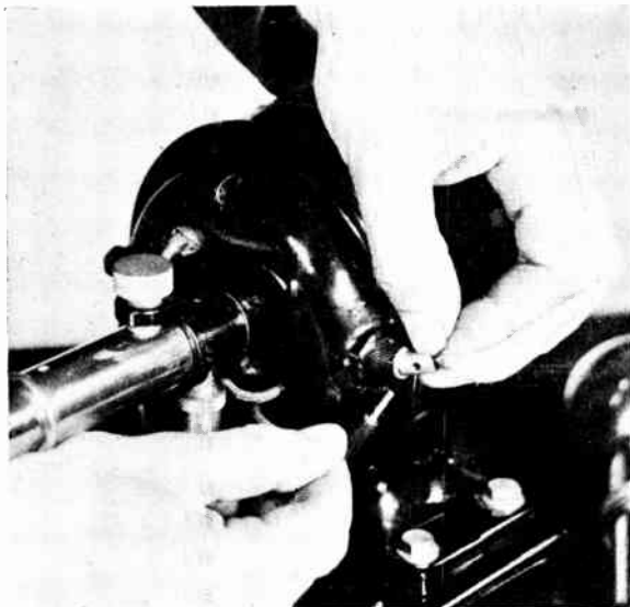
Fig. 2.—METHOD OF SECURING BRUSH IN POSITION.
