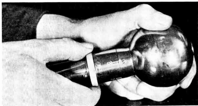
Fig. 3.—ADJUSTING THE APPARATUS FOR VARYING INTENSITY OF VIBRATION.
