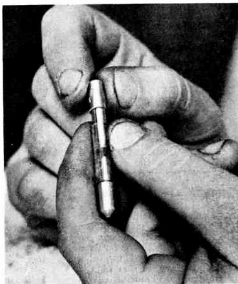
Fig. 2. —ASSEMBLING A GOLD FILM FUSE (2).
