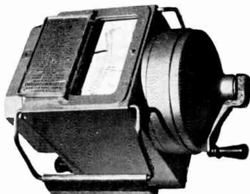
THE MEG INSULATION TESTER. ( Evershed and Vignoles, Ltd. )
