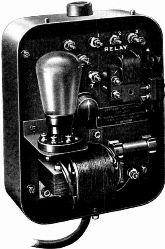
A B.T.H. PHOTO-ELECTRIC RELAY FOR INDUSTRIAL CONTROL PURPOSES.
