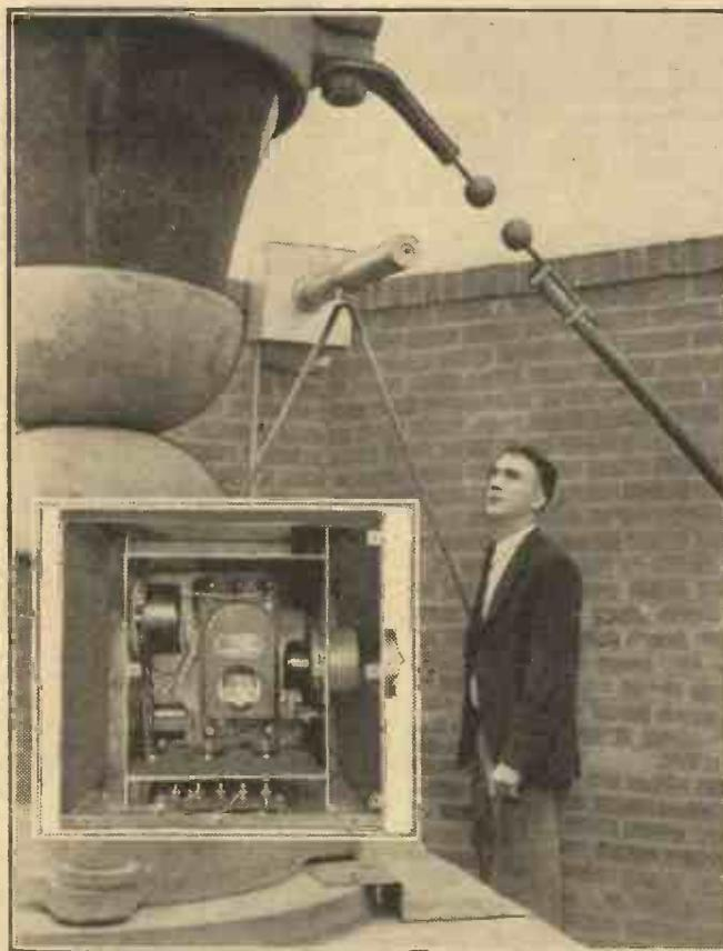
The positions of the spark-gap and the "electric eye" are shown in the large portion of this photograph, while the interior of the box containing the photo-cell gear is shown in the inset picture.
