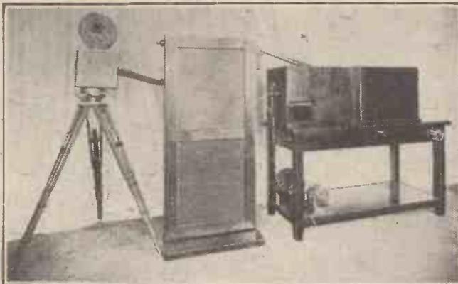
The Fernseh A.-G. Company, of Germany, partners of the British Baird Company, exhibited a new television scheme at their show. By means of this apparatus any scene can be photographed on a film, which is then automatically developed, fixed, and transmitted, all in 15 seconds! By this means events all over the country can be seen in the home almost as soon as they occur.
