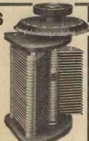
The Standard "J.B." (Illustrated) is mounted on pure ebonite end plates—hand polished, free from all surface leaks. The dielectric losses of "J.B." Condensers are negligible. Spacers are of special design; the spacing is the smallest possible consistent with practical operation; adjustment is secured by an ingenious compressing spring device. One hole fixing.
