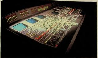
OXF-R3 AT AFS. THE DIGITAL MIXING CONSOLE COSTS AROUND £500.000 AND INCORPORATED ADVANCED CHIP SPECIFICALLY FOR THIS PROJECT
