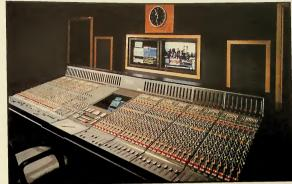
SOLID STATE LOGIC WILL BE SHOWING THE AXIOM DIGITAL PRODUCTION SYSTEM WHICH IS A TOTALLY DIGITAL RECORDING AND MIXING SYSTEM
