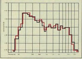
Here's a chart showing frequency spectrum analysis of the **PCM F1 digital master** of part of a recording, compared with a **pre-recorded Chrome cassette** of the same passage. The cassette was duplicated at high-speed at  $120\mu s$  normal equalisation.
