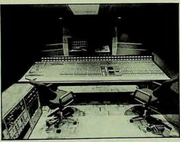
ODYSSEY STUDIO 2 control room with the recently installed SSL 6000E console. It is designed as a LEDE room which in essence enables a small room to sound like a much larger one. The creation of a non-fatiguing monitoring environment was brought about by the use of quadratic residue diffusors for the first time in Europe. Odyssey Two was the first room in the country designed and completed with the assistance of
