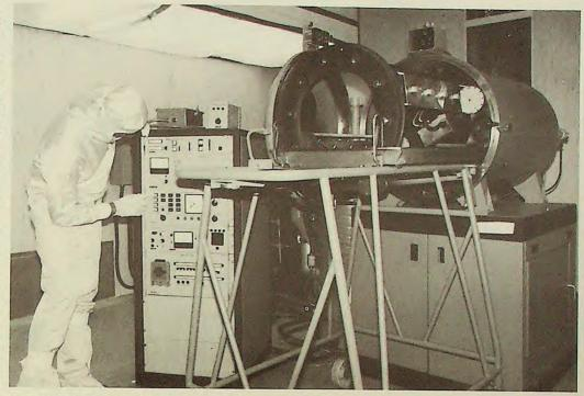
The vaporizing chamber which applies the reflective coating
