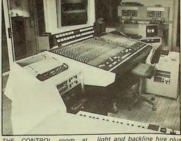
CONTROL room at IHE CONTROL room at E-Zee Studios, London. Equipment includes a Rebis Omega 30-24 console (48 track remix), Optimix computer mixdown facility, Otari MIR 90 Mk II tape machine, Ampex ¼" + ½" 15+30 ips mastering and a wide range of outboard facilities. Fair-
