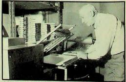
BEFORE LEAVING the premises each Hokushin cassette is carefully packaged and shrink-wrapped for protection.
