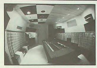
"SUPER BEAR . . . Pride of place in the control room is an MCI JH-500 automated console equipped with 28 input channels, 32 outputs and plasma display monitoring. Tape machines are also by MCI: track laying is handled by a JH-16 Series 24-track with varispeed, and two 2-track and one 4-track are on call for mastering."
