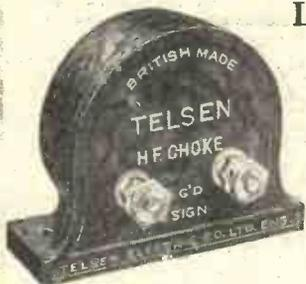
**TELSEN H.F. CHOKE.** Designed to cover the whole wave-band range, from 18 to 4,000 metres. Extremely low self-capacity. Impregnated in Genuine Bakelite. Inductance 150,000 microhenries, resistance 400 ohms. Price 2/6 each.
