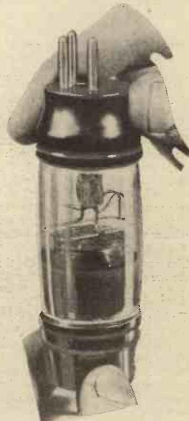
The new S.625 valve has a novel appearance. The three pins at one end are for grid and filaments, while at the other are two well-spaced pins connected to the anode and the shielding "grid." Circuits employing this valve have to be heavily screened.
