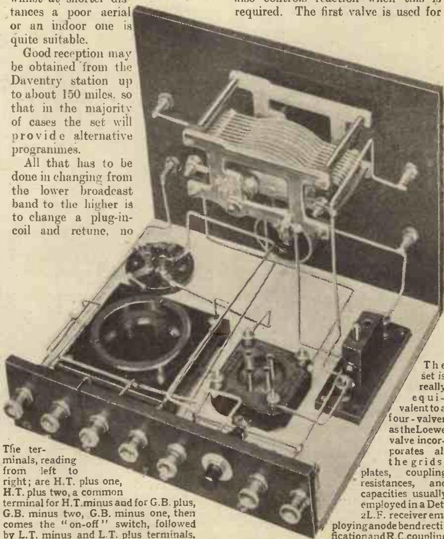
The terminals, reading from left to right; are H.T. plus one, H.T. plus two, a common terminal for H.T. minus and for G.B. plus, G.B. minus two, G.B. minus one, then comes the "on-off" switch, followed by L.T. minus and L.T. plus terminals.
