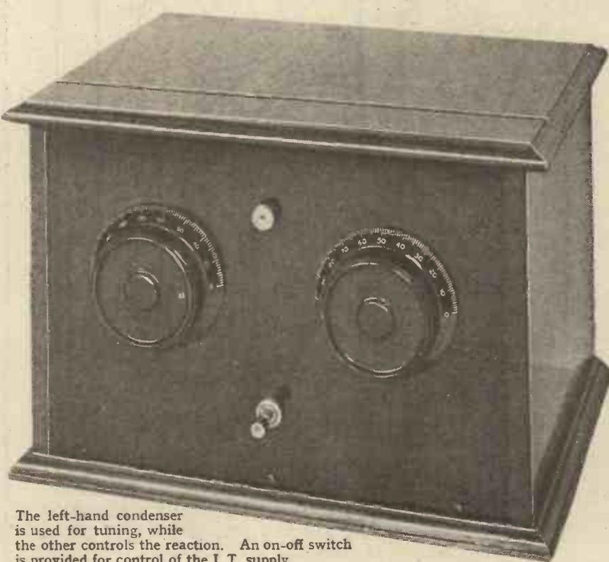
the 2-volt, but this circuit will work quite well on 4-volt or 2-volt valves provided types are chosen which suit low-frequency amplification.
