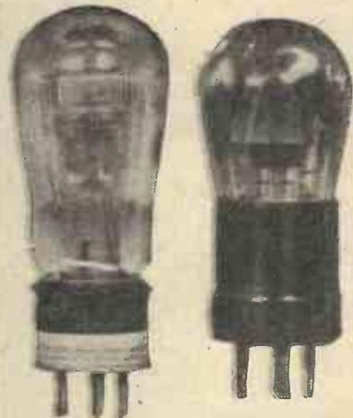
Two L.F. valves. The bright emitter C.A.C., and (right) the Stentor Two, a useful last stager.
