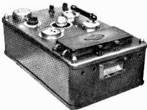
FIG. 37. IGRANIC LOW TENSION SUPPLY UNIT
