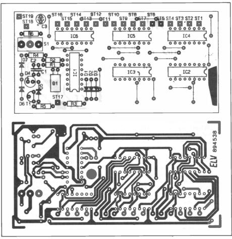
Figure 4. Printed circuit board for the transmitter.
