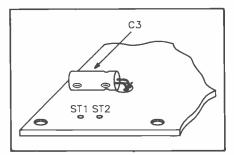
Figure 7. Mounting capacitor C3.
