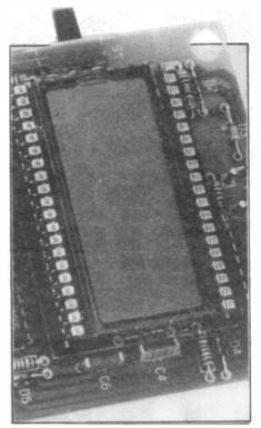
Photo 4. How the contact strips are used for the LCD.
