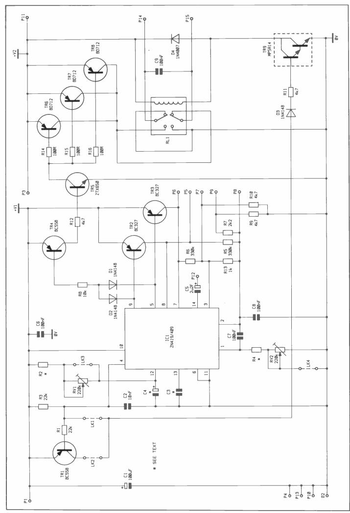
Figure 2. Combined circuit diagram of module.
