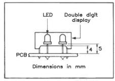
Figure 4. Inserting LD1, LD2 and DY1-4.
