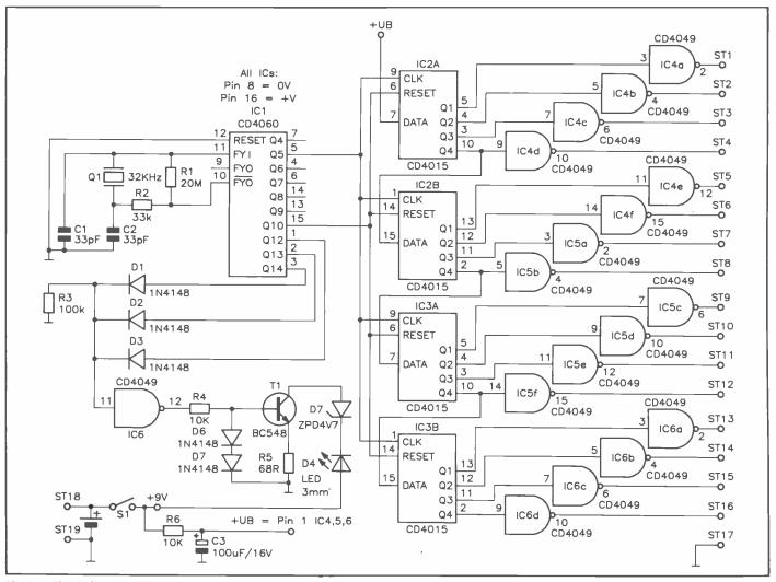
Figure 1. Circuit diagram of the transmitter unit.
