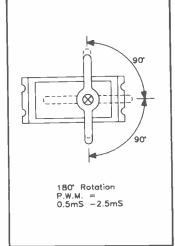
Figure 7. Servo operation.
