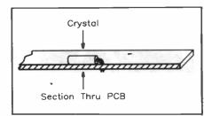
Figure 6. Mounting the crystal Q1.
