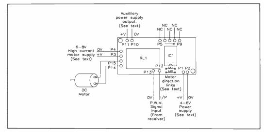
Figure 10. Motor speed control wiring diagram.
