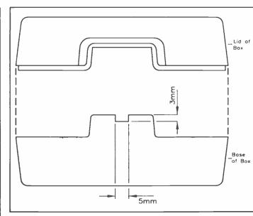
Figure 11. Receiver box cut-out details.
