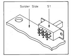
Figure 9. Mounting the receiver's on/off switch.
