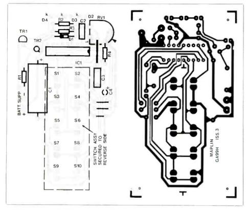
Figure 3. Component Overlay for Transmitter PCB.
