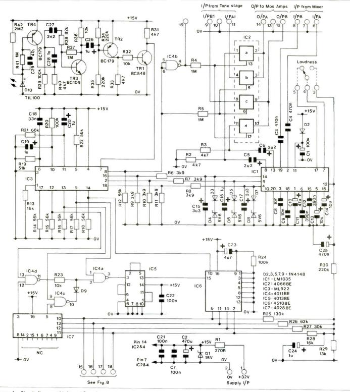
Figure 4. Circuit diagram of Infra-red Decoder.
