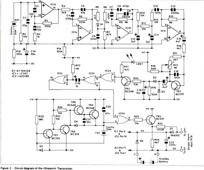
Figure 1. Circuit diagram of the Ultrasonic Transceiver. 24
