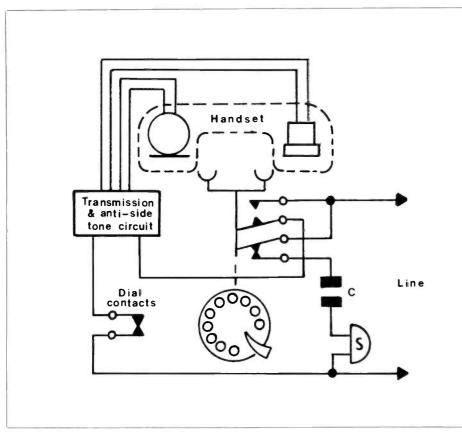
Figure 1. Block diagram of a typical telephone.
