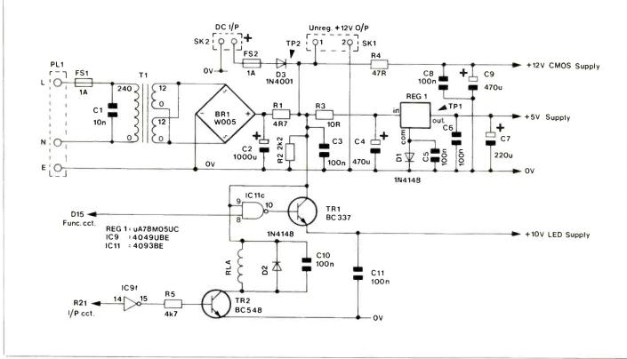
Figure 8. Power supply circuit. 32
