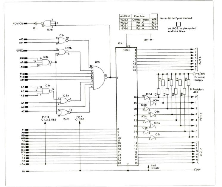
Figure 1. Circuit diagram of I/O Port.
