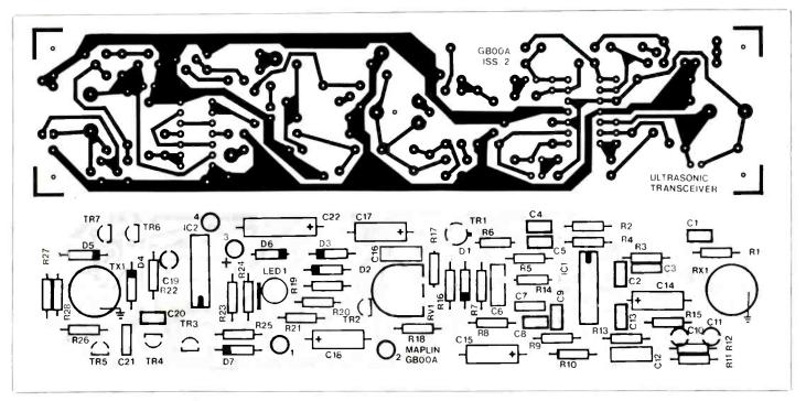
Figure 2. Component layout of the Ultrasonic Transceiver.
