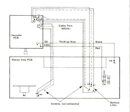
Figure 6. Connecting to 25W Mosfet Amplifier.
