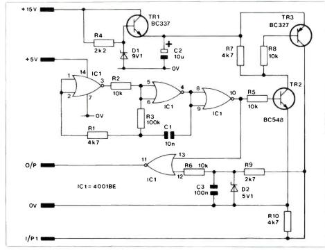
Figure 3. Circuit diagram of the Ultrasonic Interface.
