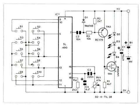
Figure 2. Circuit diagram of Transmitter.
