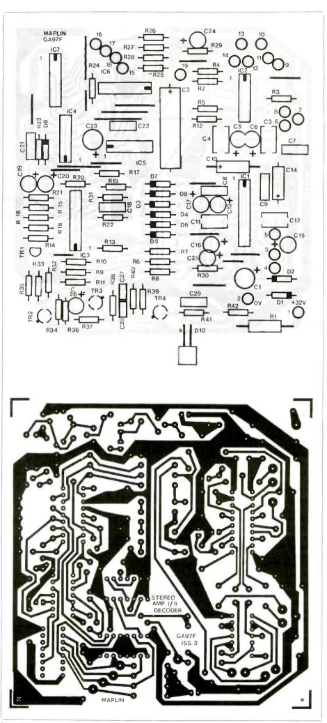
Figure 5. Component Overlay for Infra-red Decoder PCB.
