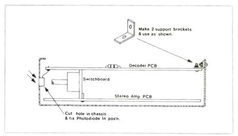
Figure 7. Mounting Decoder in 25W Mosfet Amplifier.
