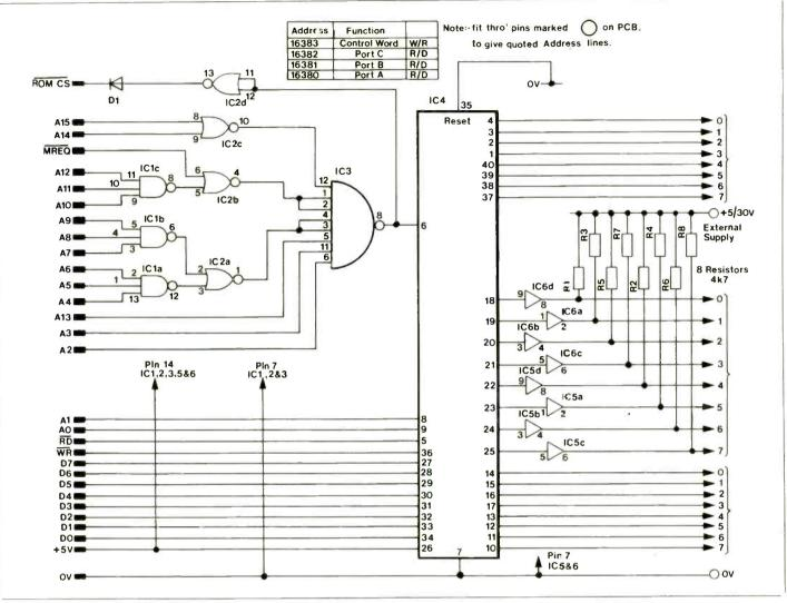
Figure 5. Circuit diagram of I/O Port with alternative address decoding.
