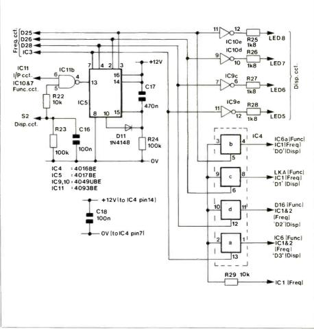
Figure 4. Gate time circuit.
