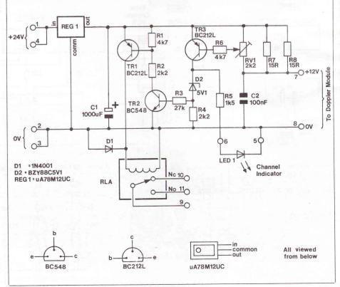
Figure 3. Circuit diagram of Extra Channel PCB.
