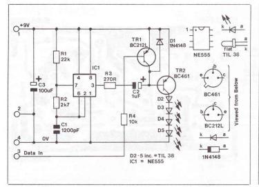
Figure 9a. Circuit diagram of Infra-red transmitter.
