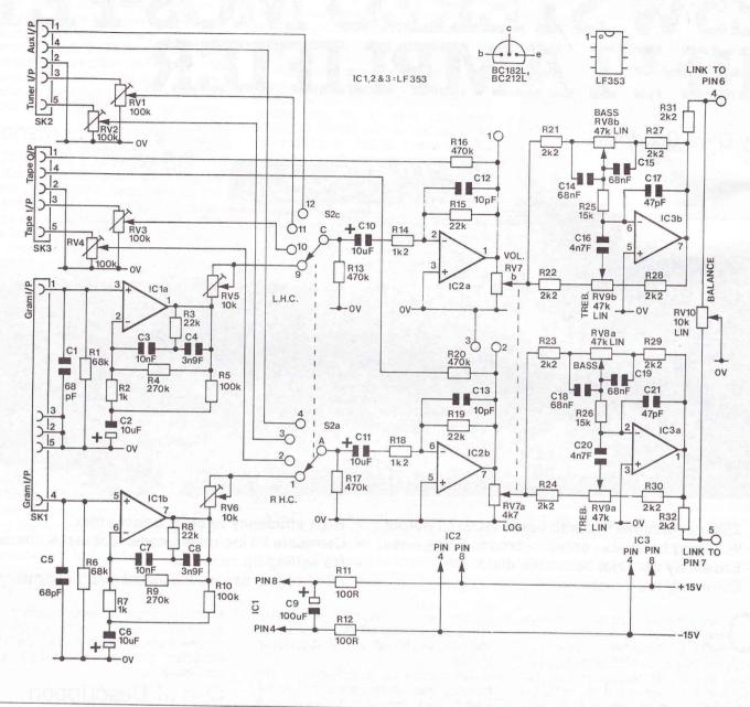
Figure 2. Circuit diagram of pre-amp and tone controls.
