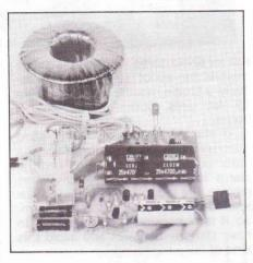
Bolt the 3-way connector block to the pcb using two 6BA ¼in bolts and nuts, then bolt the fuseholder to the pcb using a 6BA ¼in bolt and nut. LED1 and LED2 can now be connected as shown in Figure 4. These can be mounted directly to the pcb or externally depending on your requirements. LED2 shows that power is on and must be included if standby batteries are used. LED1 is used during testing, but can be omitted in use. If fitted, it lights when a Doppler module is connected.
