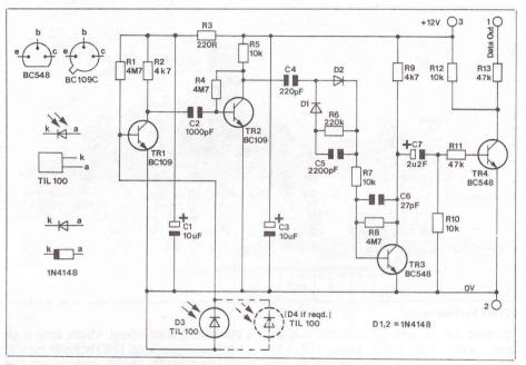
Figure 10a. Circuit diagram of Infra-red receiver.
