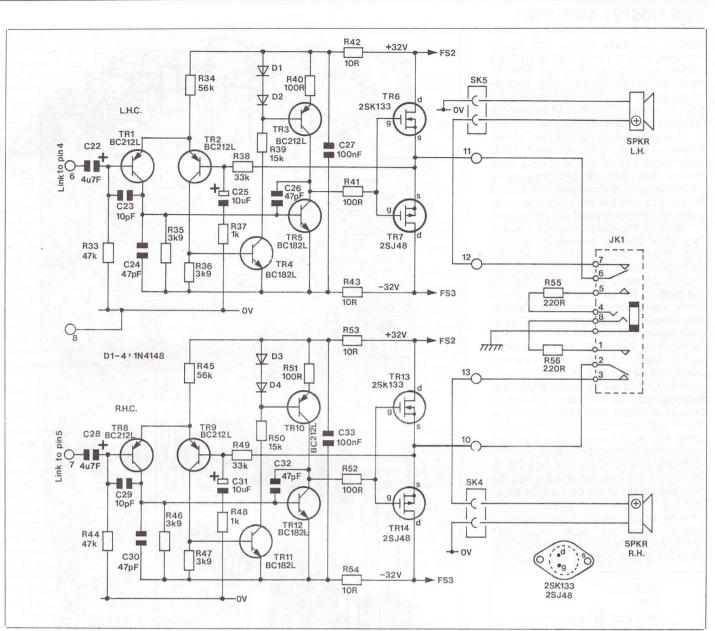
Figure 3. Circuit diagram of MOSFET power amp.
