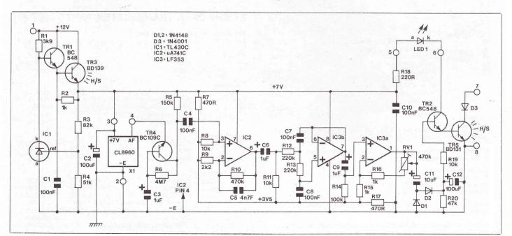
Figure 1. Circuit diagram of Doppler unit.
