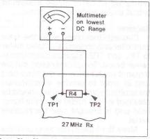
Figure 8b. Meter connections for receiver alignment.
