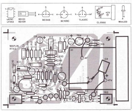
Figure 2. Component overlay of Doppler unit.
