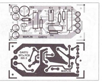
Figure 9b. Component layout of Infra-red transmitter board.
