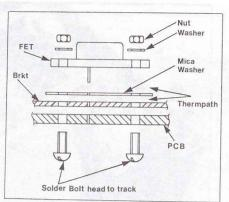
Figure 5. Mounting the MOSFET transistors.
