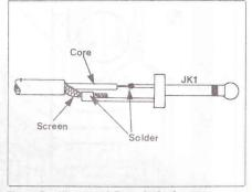
Figure 5. Wiring of 3.5mm jack plug.
