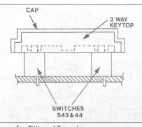
Figure 4. Fitting of 3-way key cap.
