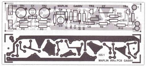
Figure 10b. Component layout of Infra-red receiver board.
