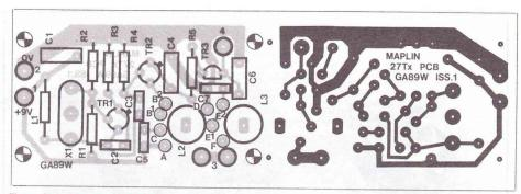
Figure 6c. Component layout of 27MHz transmitter board.
