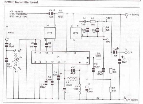
Figure 7a. Circuit diagram of 27MHz receiver.
