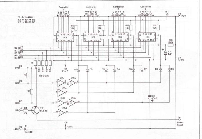
Figure 3a. Circuit diagram of Latch board.
