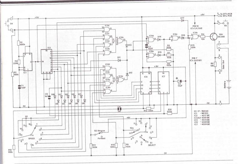
Figure 4a. Circuit diagram of Encoder board.
