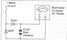
Figure 8a. RF monitor for transmitter alignment.
