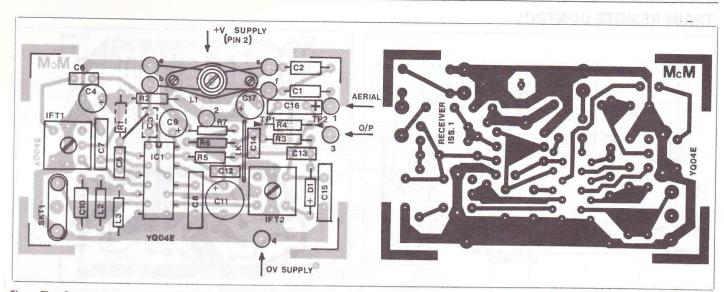
Figure 7b. Component layout of 27MHz receiver board.
