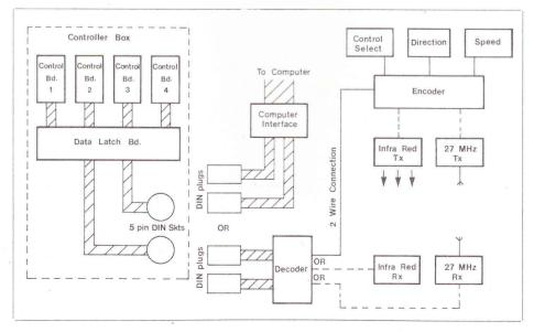
Figure 1. Block schematic showing all options.
