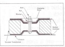
Figure 11. Mounting the toroidal transformer.
