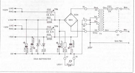
Figure 1. Circuit diagram of power supply.
