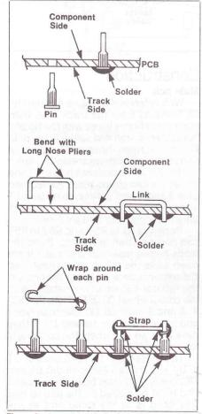
Figure 4. Insertion of pins and links in pcb. 24
