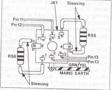
Figure 8. Jack socket wiring.
