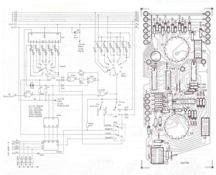
Figure 2a. Circuit diagram of complete Control board.
