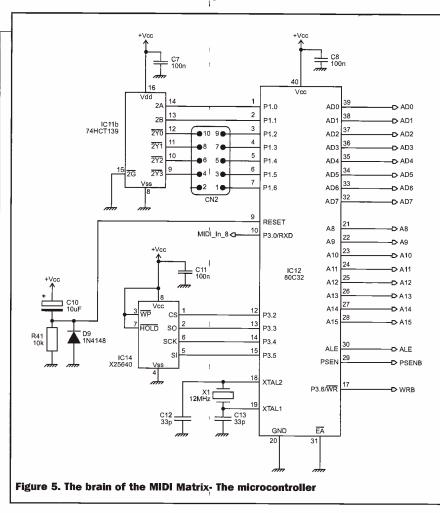
is shown in Figure 5. R41, D9 and C10 provide a power-on reset pulse to the reset input of the microcontroller, IC12. The non-volatile EEPROM connects to the microcontroller through four dedicated pins. Both the Write Protect and Hold , functions are not used in this circuit, and are wired high. The processor's clock is generated by X1, with C12 and C13 providing the correct loading for the crystal, ensuring stable oscillation and guaranteed start-up behaviour.
