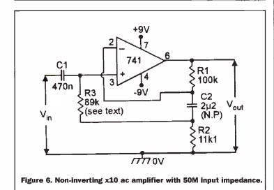
This shows a x10 amplifier. The voltage gain is determined by the ratios of R1 and R2, as indicated. If R1 is given a value of zero, the gain falls to unity; alternatively, if R2 is given a value of zero, the gain equals the open-
