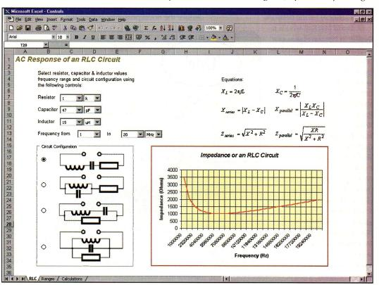
the value and units selected. Much the same procedure, but with different lists of values and units, is used for the capacitance, inductance and for the lower and upper limits of the frequency range.
