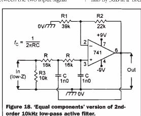
frequency ( $f_C$ ) of  $\frac{1}{\sqrt{\pi}}$  RC), and then falls at a rate of 6dB/octave (= 20dB/decade) as the frequency is increased (see Figure 16(b)). Thus, a simple 1kHz filter gives roughly 12dB of rejection to a 4kHz signal, and 20dB to a 10kHz one.
