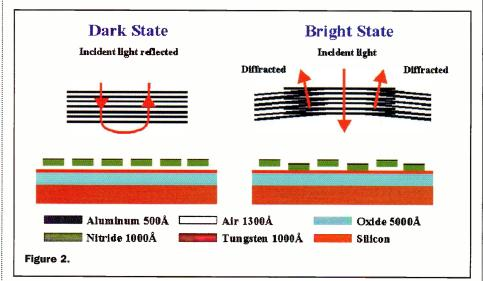
diffraction produces light at a different angle to that of the incident light and it passes out (see side view Figure 2).
