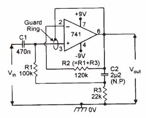
Figure 9. Ac voltage follower with 50M input impedance without the guard ring, or 500M with the guard ring.
