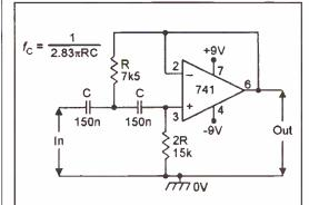
Figure 20. Unity-gain 2nd-order 100Hz high-pass filter.
