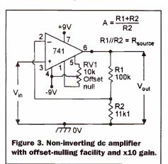
gain of x100, the output may be offset by 100mV with zero input applied. Also note that the circuit's bandwidth equals the  $f_T$  value (typically 1MHz in a 41) divided by the 'A' value, e.g., the Figure 1 circuit gives a bandwidth of 100kHz with a gain of x10, or 10kHz with a gain of x100.
