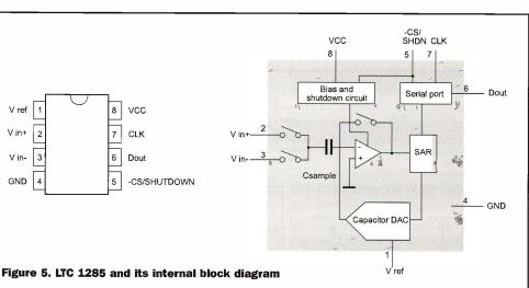
initiated at the falling edge of the chip select -CS/SHDN (pin 1). After -CS falls the second CLK pulse enables Dout. A null bit (logic 0) appears on the Dout (pin 6) firstly. At the next 12 falling edge of the clock, the 12 bits of the A/D conversion result appear on Dout one by one.
