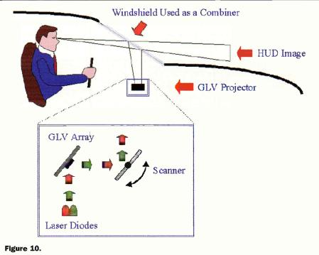
advantages of this approach are that an HDTV image of 1920x1080 pixels only requires a 1080-pixel column instead of over two million pixels of an area array much reducing the bandwidth; the aspect ratio can easily be changed; and the
