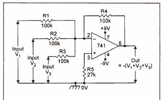
Figure 12. Unity-gain inverting dc adder.
