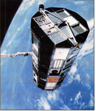
NASA photograph of the Long Duration Exposure Facility. Space exploration must be one of the most demanding applications for electronic circuitry. The LDEF shown here has been used, among other applications, for investigating the effect of long exposure to space on electronic equipment. Photo courtesy NASA
