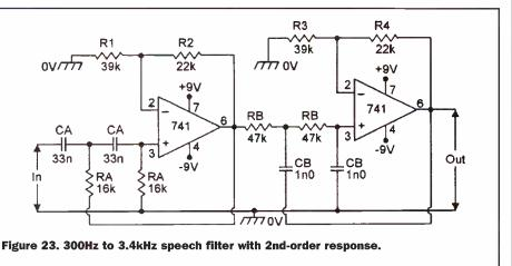
Note here that the op-amp is designed to give a voltage gain (4.1dB in this case) via R1 and R2, which must have the values shown.
