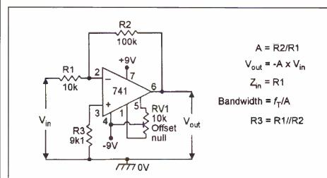
Figure 1. Inverting dc amplifier with offset-nulling facility and x10 voltage gain.
