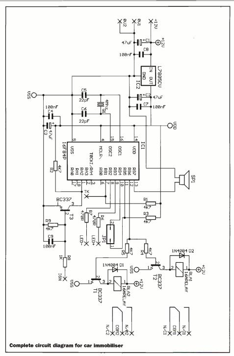
it that the ignition is switched on or off. The two output relays are heavy duty relays, primarily intended for automotive applications. The contacts are rated at 16 amps, 24v DC, and each relay has a N/O and N/C contact. The relays are activated via T1 and T2. The TK input is connected to the touch key receptacle, and is used to communicate with the touch key.
